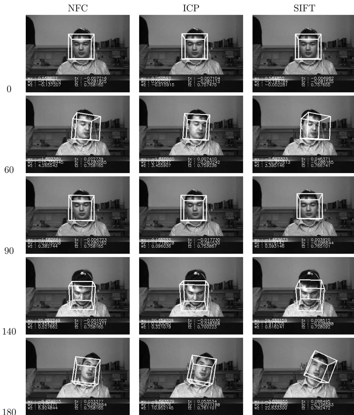
Figure 5.9: Head tracking results for time varying illumination change sequence 1. Each row represents tracking results at different frames: 0, 60, 90, 140, 180
