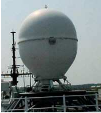
Figure 3.6 CAS Fire Control Radar [29]
