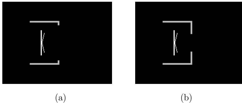
Figure 3.1: (a) Transducer with the real dimensions, (b) Transducer modified for desired directivity pattern
