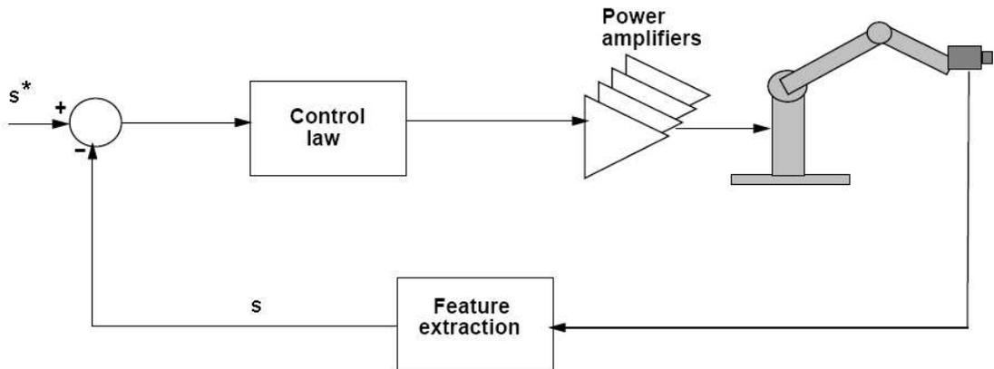
Figure 2.9: Image based direct visual servoing
