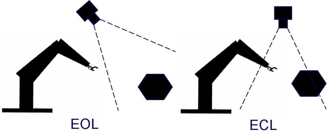
Figure 2.4: Endpoint open-loop and endpoint closed-loop systems
