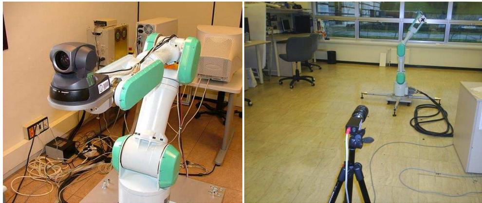
Figure 2.2: Eye-in-hand and eye-to-hand configuration on PA10
