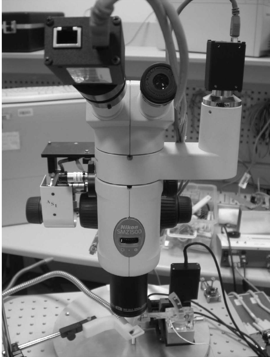
Figure 5.14: Microassembly workstation and attached visual sensors
