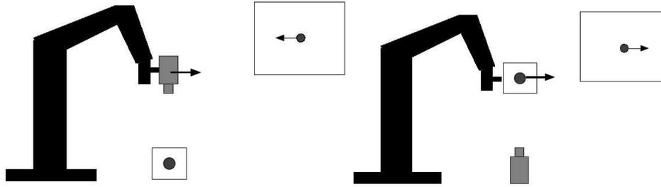
Figure 2.1: Eye-in-hand and eye-to-hand camera configurations
