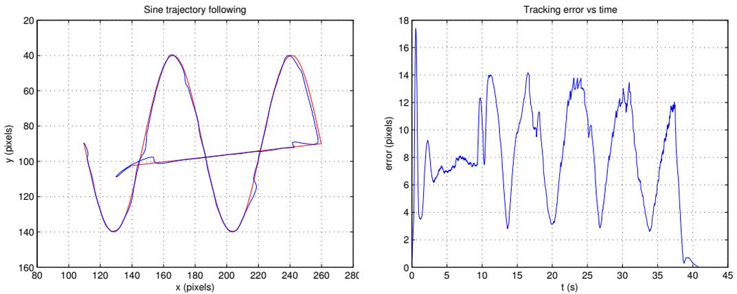
Figure 5.13: Sine trajectory and tracking error for dynamic Gauss-Newton controller with RLS Jacobian estimation
