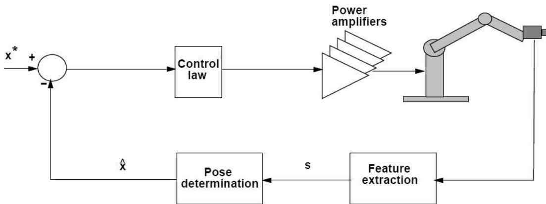
Figure 2.7: Position based direct visual servoing
