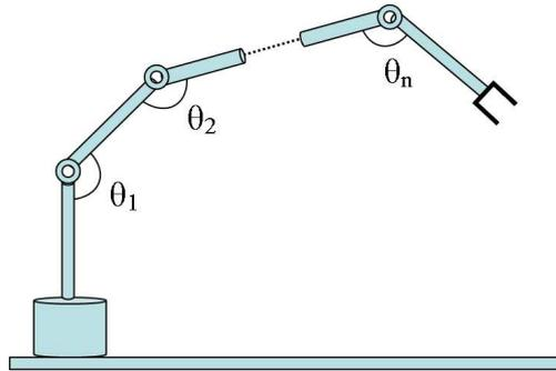
Figure 3.1: Joint variables of a robot
