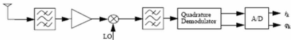
Figure 2.2 Common Transmitter Architecture
