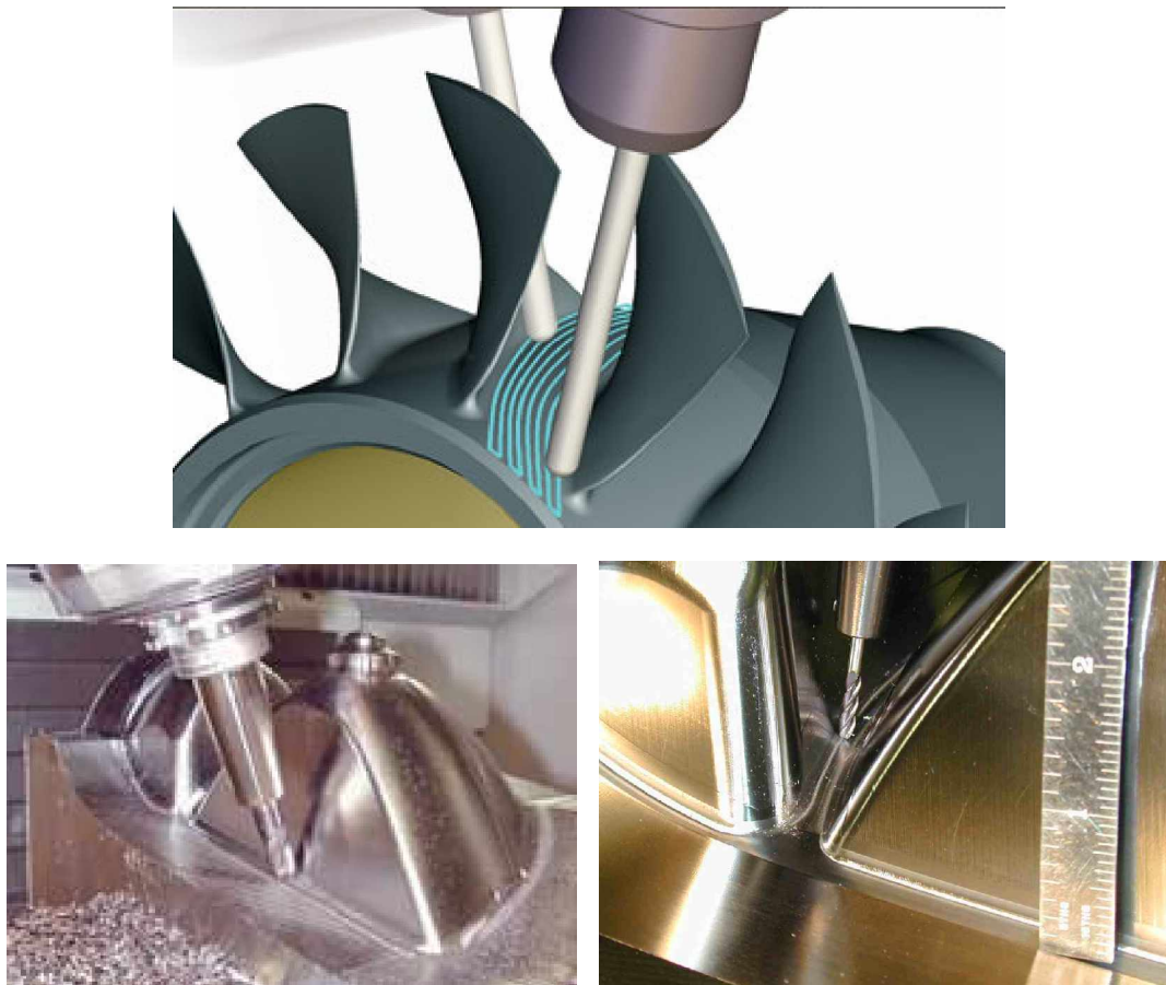
Figure 1-4: Workpiece – cutter interaction in 5-axis milling
