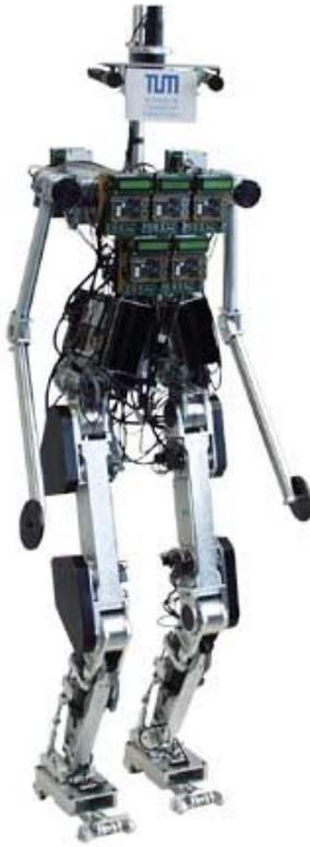
Figure 3.4. Humanoid robot Johnnie of the University of Munich.
