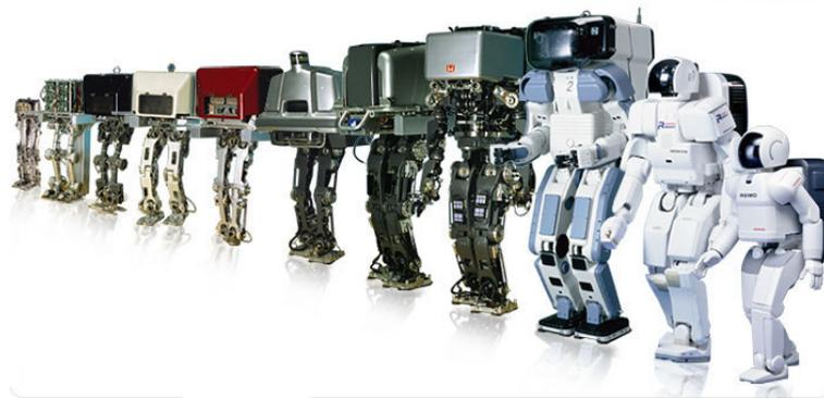
Figure 3.1. All the robots from Honda's humanoid project since 1986.
