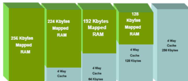
Figure 3.5: Partitioning internal memory into L2 cache/ram
