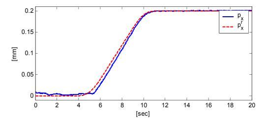
Figure 7.4. 0.2mm reference trajectory for  $p_x$  and measured motion
