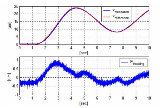
Figure 3.11. Response to a varying amplitude sine reference
