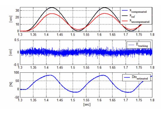
Figure 4.4. Response to  $u_0 = 30\sin(10\pi t) + 30$  with disturbance compensation
