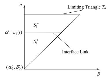
Figure 1.3. Monotonically increasing input  $u_1(t)$
