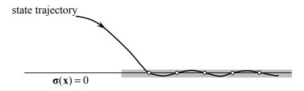
Figure 2.3. Discrete-time Sliding mode in sampled-data systems
