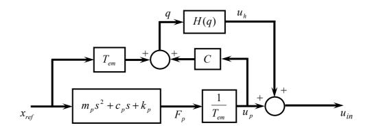
Figure 3.8. Inverse model of the PZT actuator
