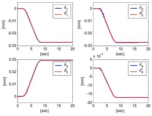
Figure 7.8. Reference limb trajectories for  $0.1 \text{mm } p_x$  trajectory
