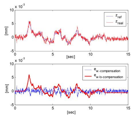
Figure 5.12. Dual-stage 1.5mm sigmoid reference tracking (contd.)
