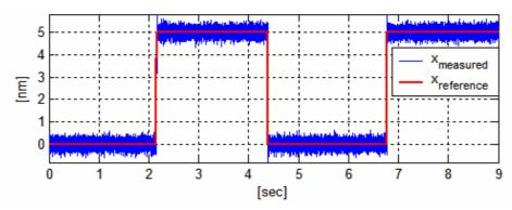
Figure 4.12. 5nm step motion
