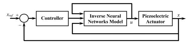
Figure 1.4. Closed-loop neural network controller
