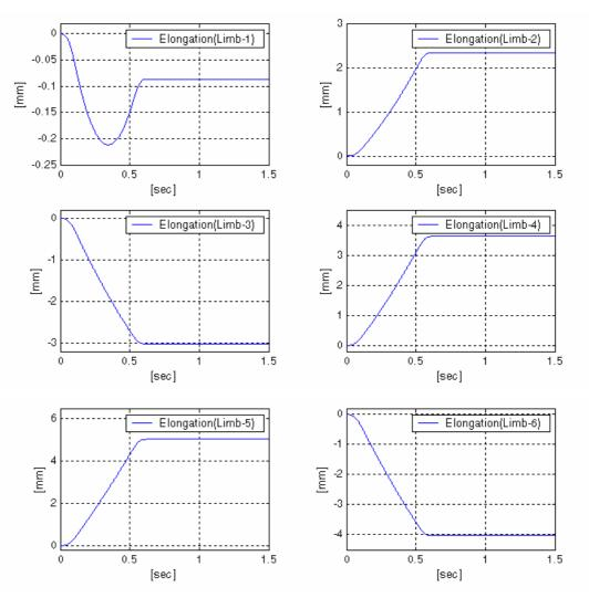
Figure 6.6. Required limb elongations for the first set of trajectories
