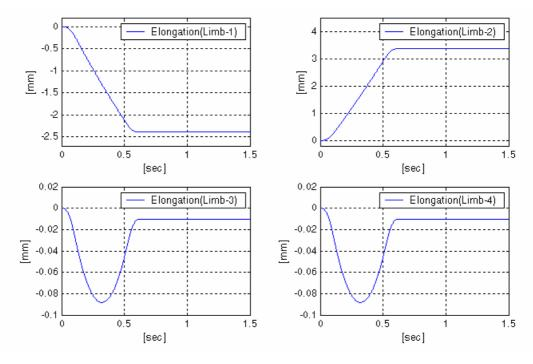
Figure 6.9. Limb elongations for the second set of trajectories
