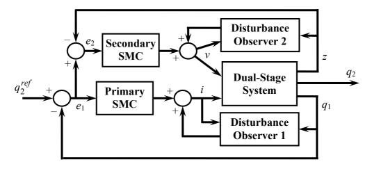
Figure 5.8. Dual-stage Controller scheme
