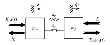
Figure 5.3. Model representation of the system
