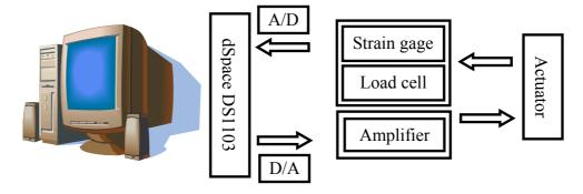
Figure 4.9. Structure of the experimental setup
