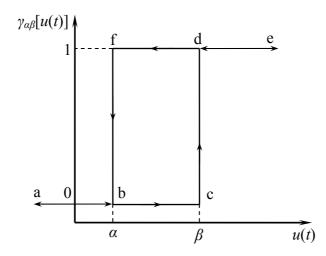
Figure 1.2. Hysteresis operator  $\gamma_{\alpha\beta}[u(t)]$
