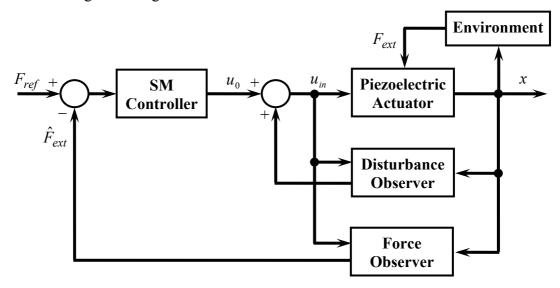
Figure 4.14. Block-diagram of force control system
