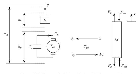
Figure 3.3. Electromechanical model of the PZT actuator, [1]
