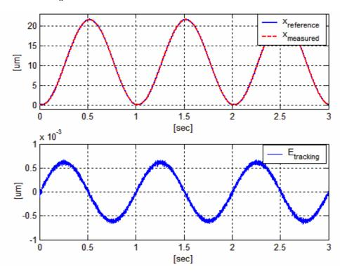
Figure 4.11. Closed-loop response to a 1Hz sinusoidal reference
