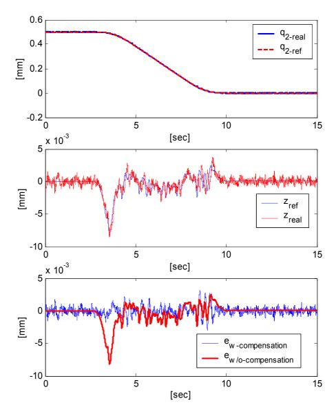
Figure 5.9. Dual-stage 0.5mm sigmoid reference tracking
