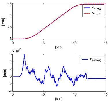
Figure 5.7. Single-stage 1.5mm sigmoid reference tracking
