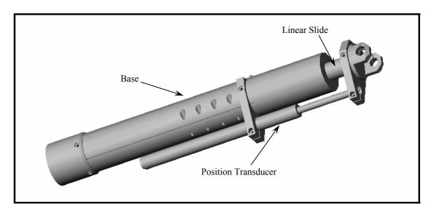
Figure 5.1. CAD model of the dual-stage system
