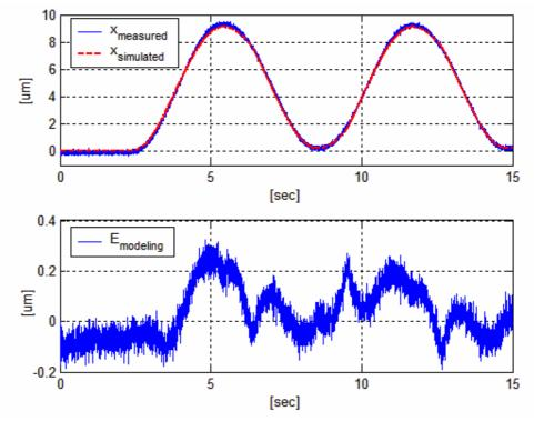
Figure 3.7. Response to  $u = 15 + 15\sin(t)$  and corresponding modeling error
