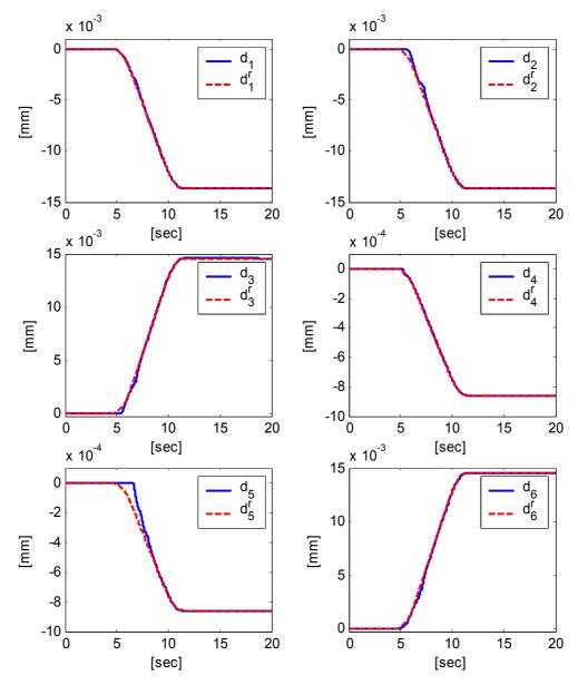
Figure 7.11. Reference limb trajectories for  $50\mu m p_x$  trajectory
