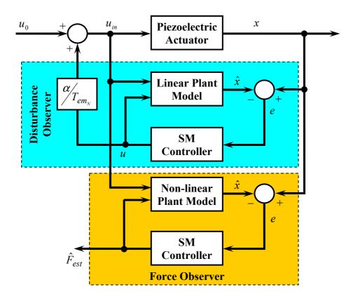
Figure 4.6. Block-diagram for external force estimation
