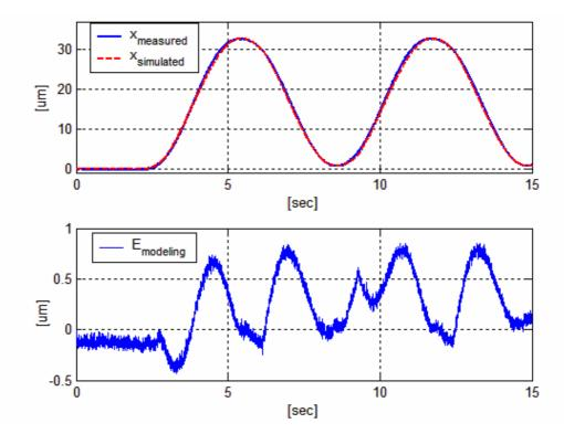
Figure 3.6. Response to  $u = 40 + 40\sin(t)$  and corresponding modeling error
