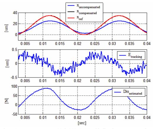
Figure 4.5. Response to  $u_0 = 30\sin(100\pi t) + 30$  with disturbance compensation
