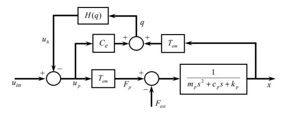
Figure 3.4. Block-Diagram representation of the electromechanical model
