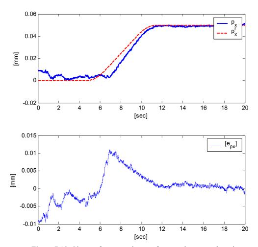
Figure 7.10. 50 $\mu$ m reference trajectory for  $p_x$  and measured motion
