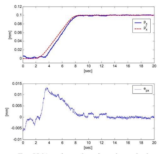
Figure 7.7. 0.1mm reference trajectory for  $p_x$  and measured motion
