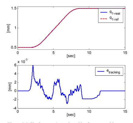
Figure 5.6. Single-stage 1mm sigmoid reference tracking
