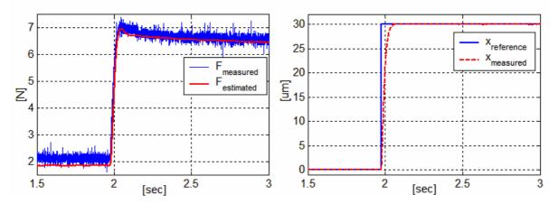
Figure 4.7. Results of the Force Observer Experiments
