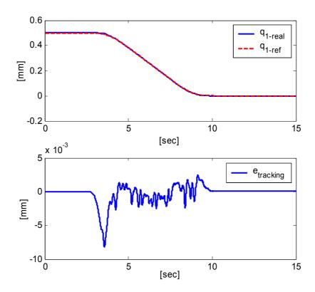
Figure 5.5. Single-stage 0.5mm sigmoid reference tracking
