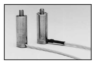
Figure 3.1. Stack actuators used in the experiments
