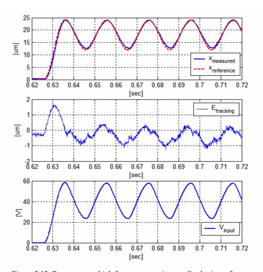
Figure 3.13. Response to a high frequency varying amplitude sine reference
