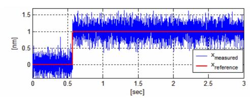
Figure 4.13. 1nm step motion
