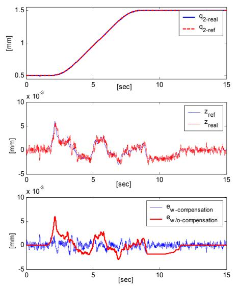
Figure 5.10. Dual-stage 1mm sigmoid reference tracking
