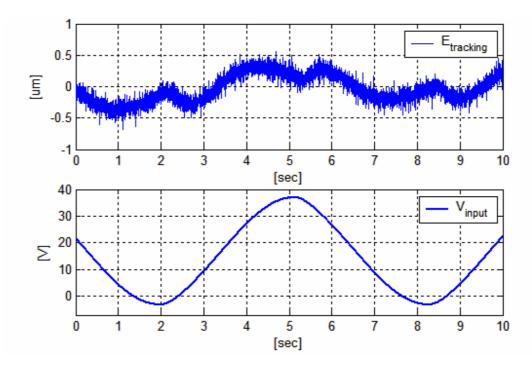
Figure 3.10. Open-loop tracking error and input voltage for  $x_r = 7.5 + 7.5 \sin(t)$
