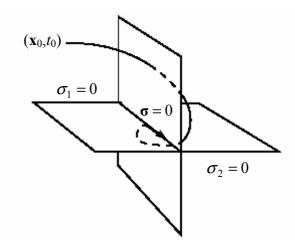
Figure 2.1. Geometric interpretation of two intersecting switching surfaces
