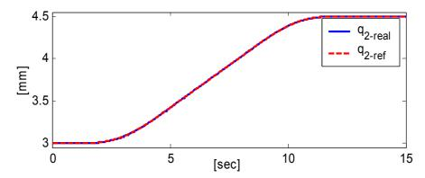
Figure 5.11. Dual-stage 1.5mm sigmoid reference tracking
