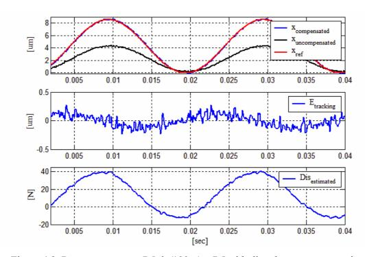
Figure 4.3. Response to  $u_0 = 7.5\sin(100\pi t) + 7.5$  with disturbance compensation
