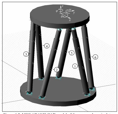
Figure 6.3. MSC.ADAMS CAD model of the proposed manipulator
