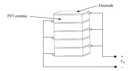
Figure 3.2. Illustration of a PZT stack actuator
