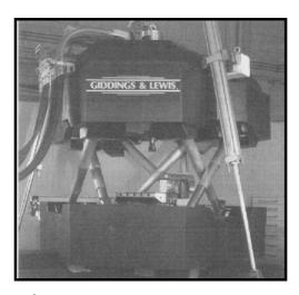
Figure 6.1. VARIAX® machining center, Giddings and Lewis machine tools
