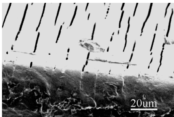
Figure 3.7 Scanning electron micrograph of APS treated Eppendorf tube taken from the cross-sectional viewpoint, tilted slightly towards the inner face
