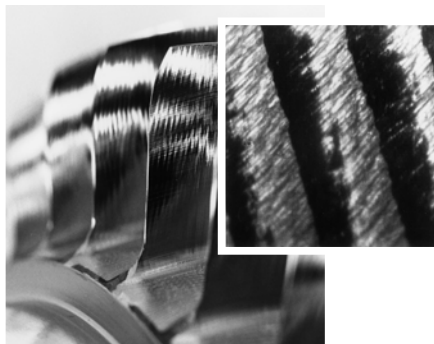
Figure 1.6: Chatter marks on the surface
