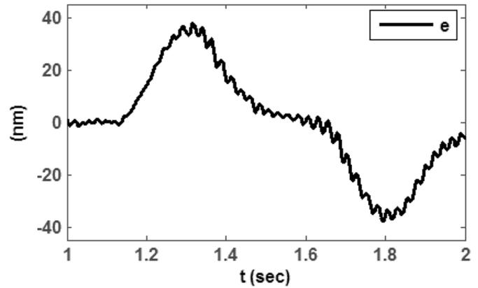
Fig. 11. Tracking performance of PID control.
