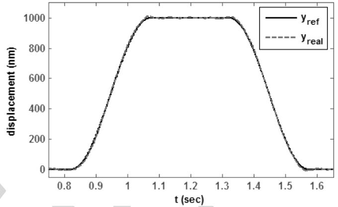
Fig. 6. Open-loop with compensation response to a trapezoidal reference.
