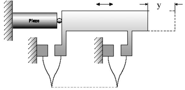
Fig. 1. Structure of a flexure piezostage.
