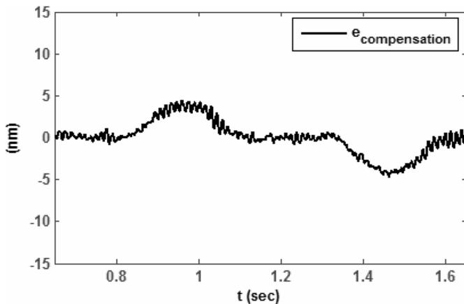
Fig. 9. Tracking performance of SMC with compensation.
