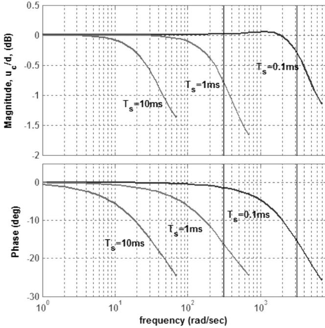
Fig. 3. Frequency response of estimated disturbance w.r.t. disturbance.
