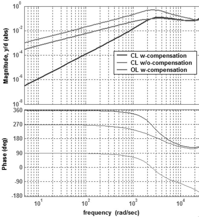
Fig. 4. Sensitivity (micrometer/volt) of the controlled position w.r.t. disturbance.
