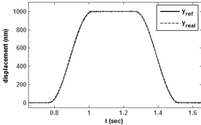
Fig. 8. Response with SMC and compensation.
