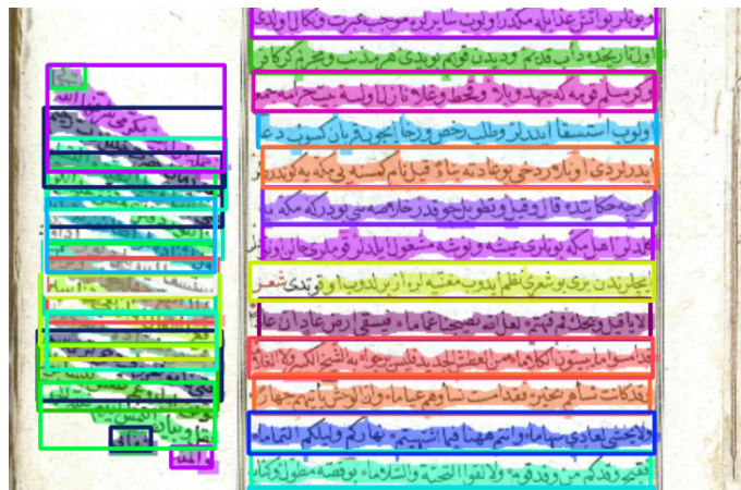
Figure 5.5 Sample output crop from the YOLO segmentation approach, illustrating how bounding boxes were used to localize text lines
