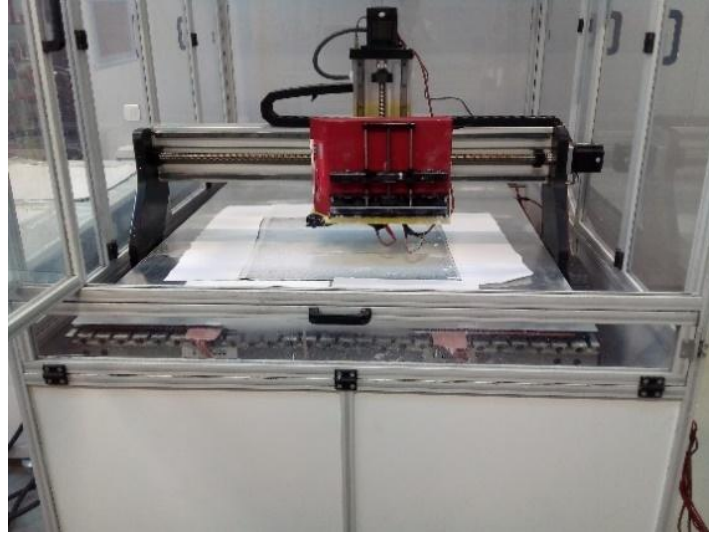
Figure 5.S1 Electrospaying set-up for the deposition of h-BN particles onto carbon fabrics.
