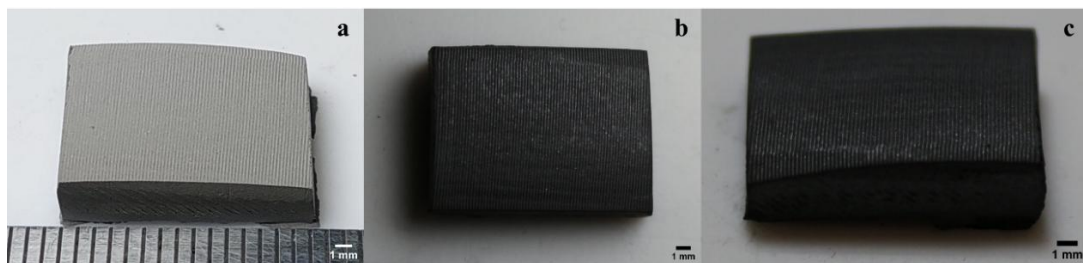
Figure 3.8. (a) Sharkskin-like texture on green body, (b-c) Views from the sintered body
