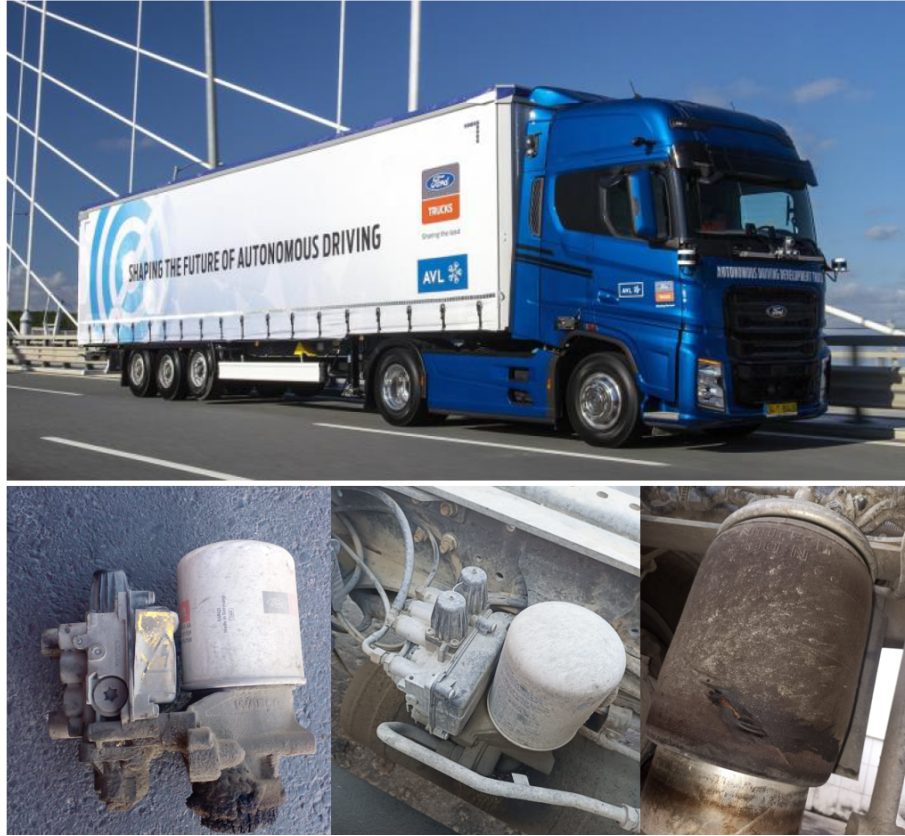
Figure 1.3 Overview of APS failures in HDVs. The top image shows a typical HDV, and the bottom displays three examples of failed E-APUs (images were adapted from Mumcuoglu et al. (2024b) and Aydemir (2024)).
