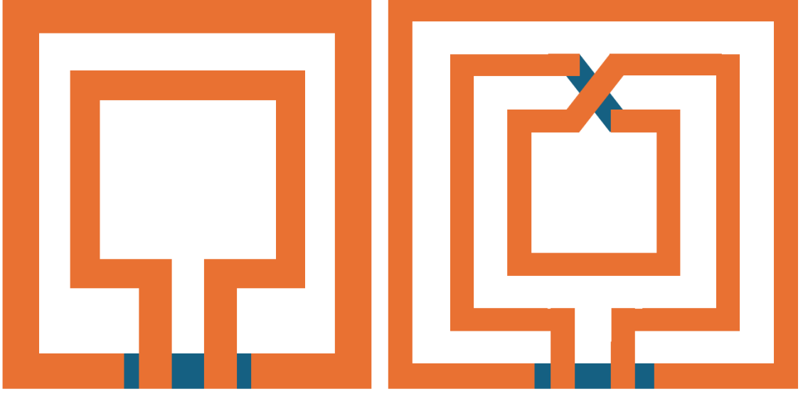
Figure 3.11 One turn and two turn square inductor layouts
