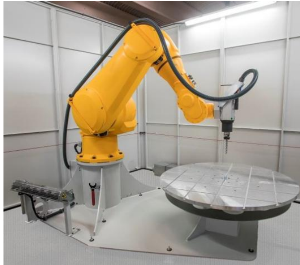
Figure 6.4 The Stäubli TX 200 industrial robot with round fixture table
