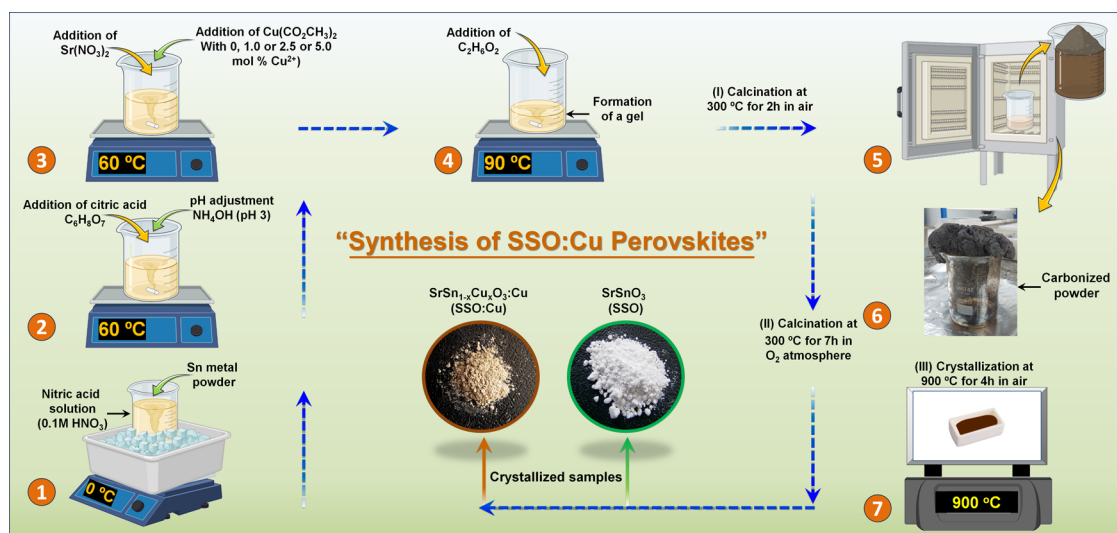
Scheme 1. Schematic Diagram for the Synthesis Procedure of the \text{SrSn}_{1-x}\text{Cu}_x\text{O}_3 (SSO:Cu _x ) Samples
