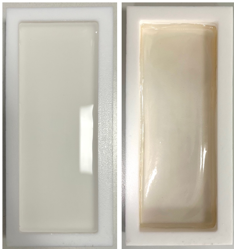
Figure 5: (left) SAP solution after polymerization, (right) solid SAP after drying.
