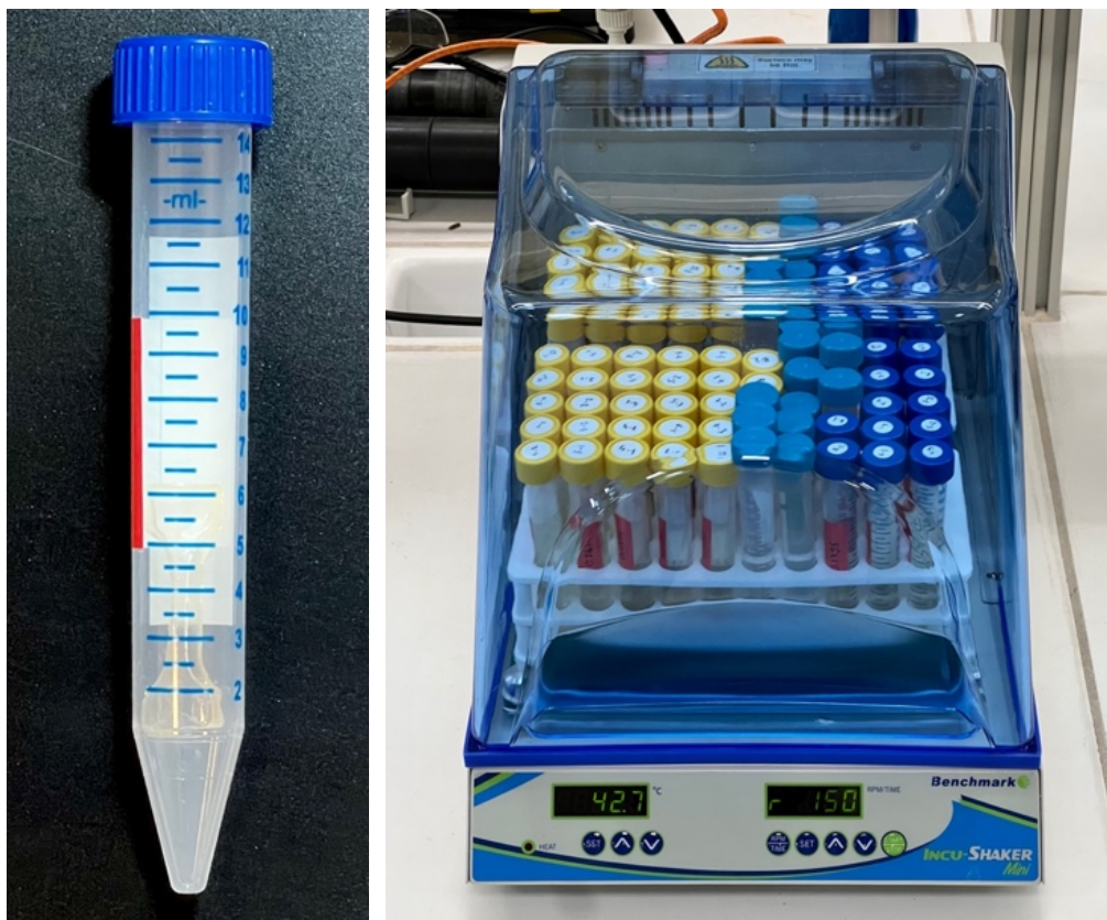
Figure 14: SAP sample in falcon tube (left), and biodegradation test setup in incubator (right).
