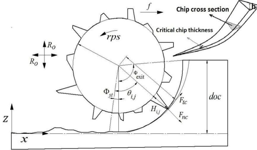
Figure 41: schematic of grinding process
