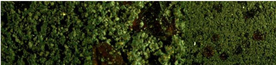
Figure 25: CBN Grits bonded with Bronze-Ti mixture, keep the furnace constant at 900°C and reduce the Ti ratio to 10%
