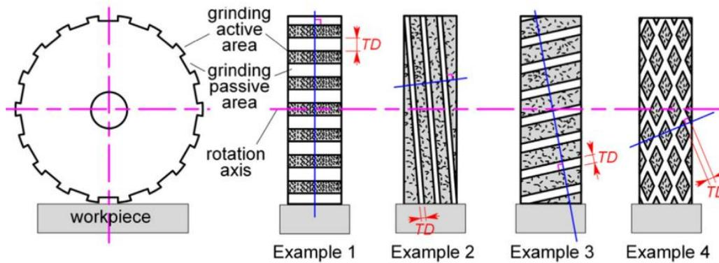
Figure 20: Schematics of possible designs of textured grinding wheels revealing the key texture dimension
