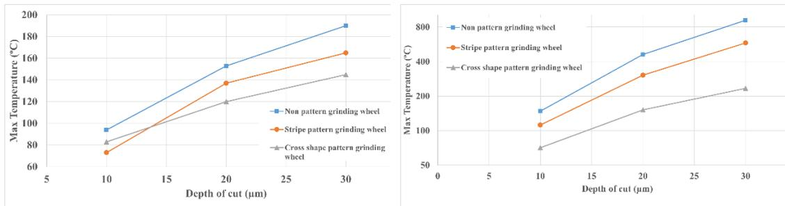
Figure 37: Temperature data for different depth of cuts, spindle speed 25000rpm and feed rate 200mm/min
