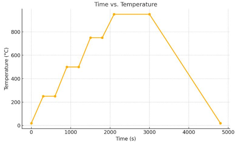
Figure 14: Brazing simulation time step, pulsed heating and cooling rate
