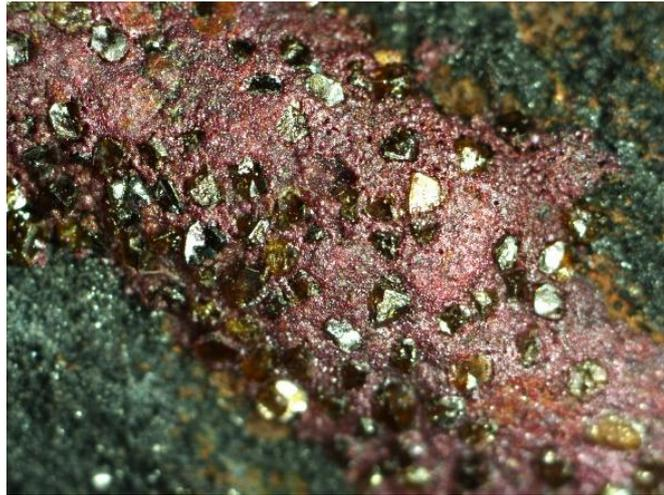
Figure 31: 5% Titanium, Overnight Cooling, Argon as Flushing Gas
