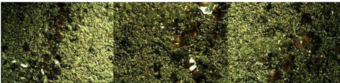
Figure 26: CBN Grits bonded with Bronze-Ti mixture, furnace brazing at 850°C and increase the Ti ratio to 10%
