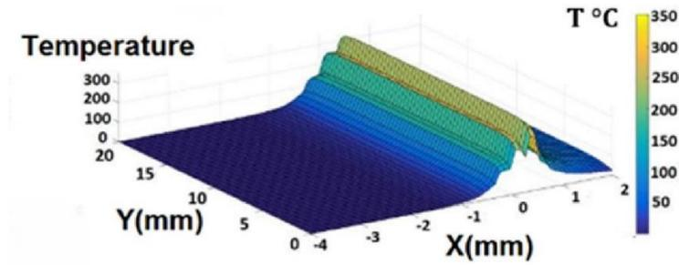
Figure 8: an Example for Generated Temperature during Grinding
