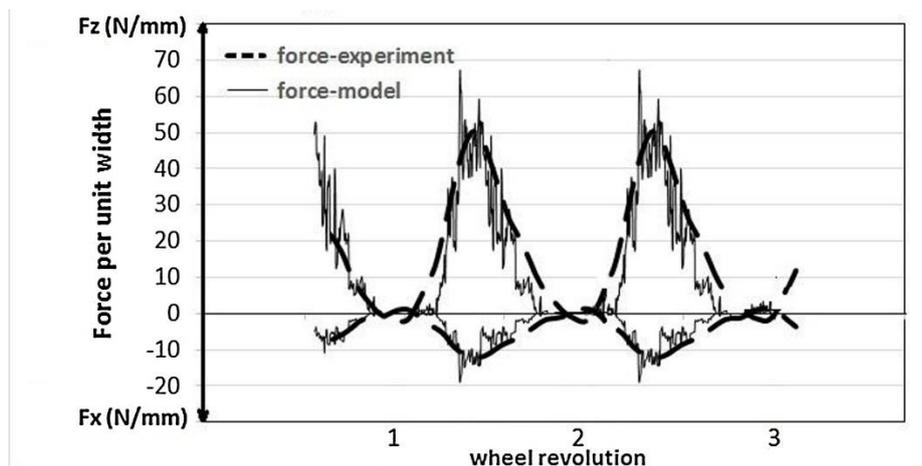
Figure 9: Total Force Profile for x and z direction
