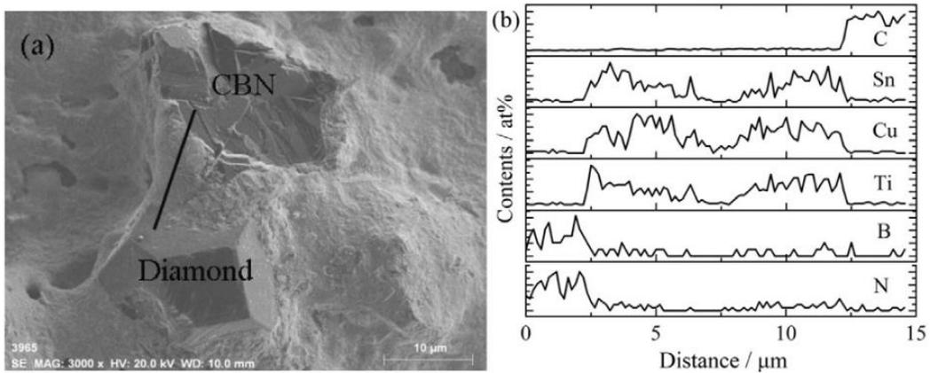
Figure 5: Microstructure of brazing interface between diamond and CBN with Cu–Sn–Ti active filler (a) SEM image, (b) elemental distribution curves of (a) [47]
