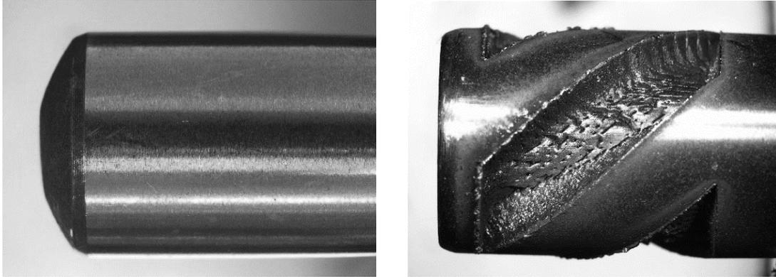
Figure 28: Raw substrate through the procedure of preparation after laser ablation
