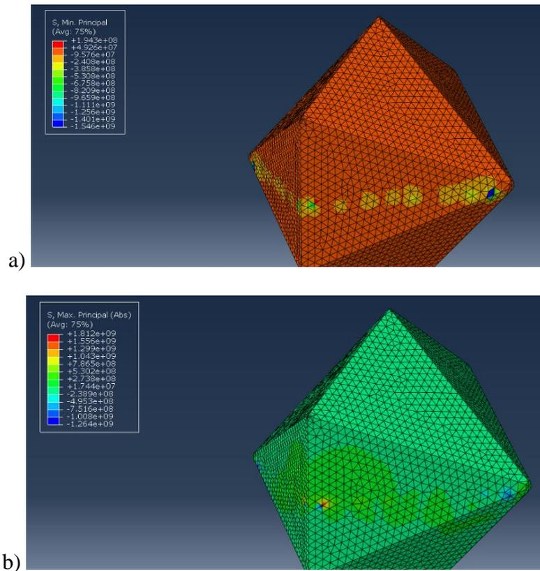
Figure 17: Maximum and minimum Principle stresses
