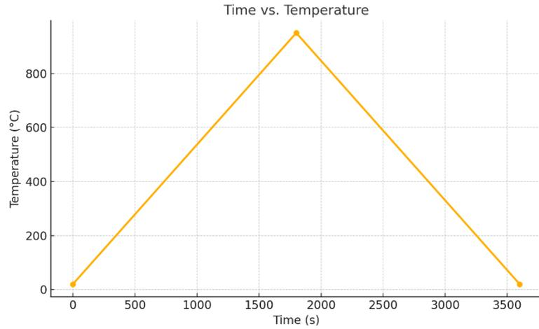
Figure 12: Brazing simulation time step, constant heating and cooling rate
