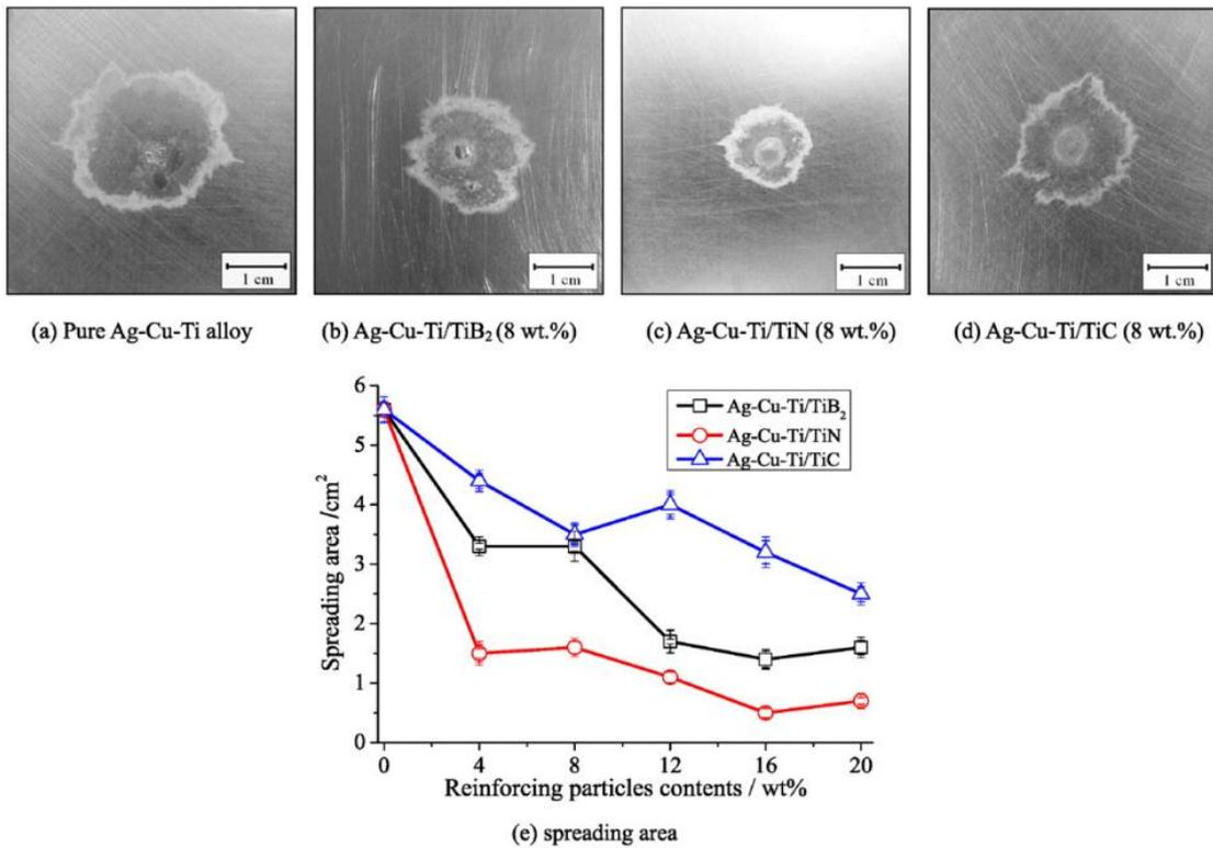
Figure 4: Effects of the reinforcing particles on the spreading morphology and area of composite filler materials [45]
