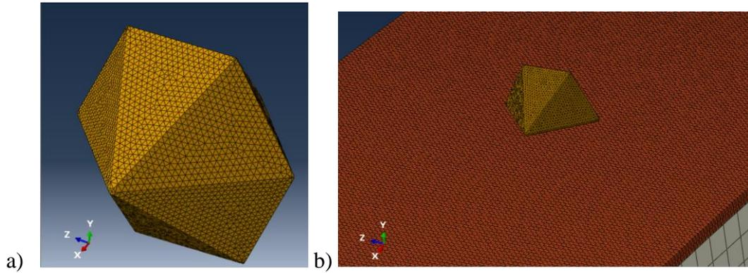
Figure 11: a) CBN grit shape demonstration b) Single Grit implementation in bonding material for Stress analysis
