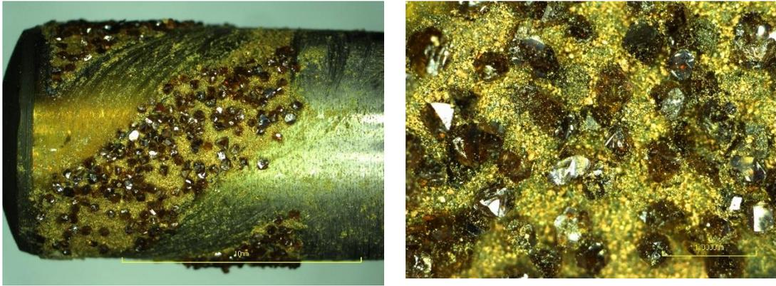
Figure 29: assembled substrate at the very last step before furnace brazing
