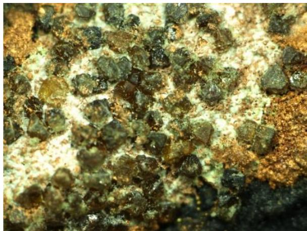
Figure 30: 7% Titanium, Overnight Cooling, Argon as Flushing Gas
