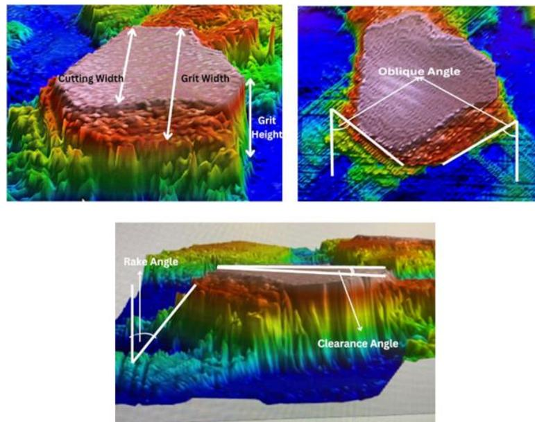
Figure 7: CBN measurements with Nanofocus
