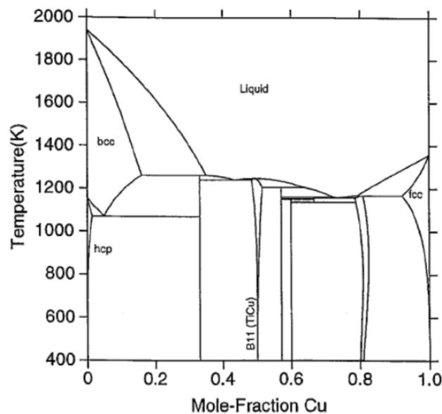
Figure 24: Ti - Cu phase diagram
