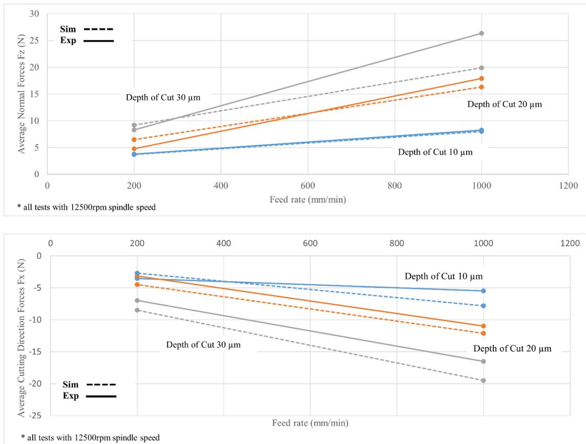
Figure 36: Simulation and experimental results for grinding forces different depth of cuts
