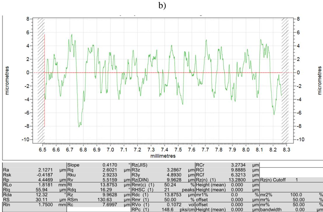
Figure 23: Sample Surface Roughness measurement,
