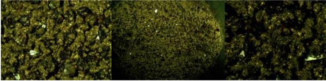
Figure 27: CBN Grits bonded with Bronze-Ti mixture, keep the furnace constant at 900°C and reduce the Ti ratio to 5%
