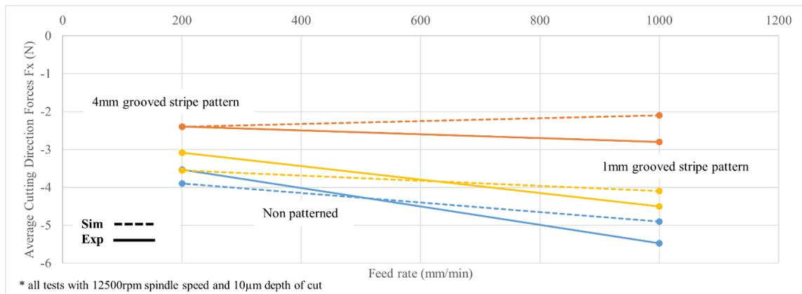
Figure 40: Force values for both simulation and experimental for comparing patterned and normal wheels
