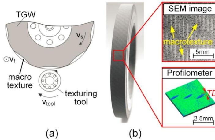
Figure 1: Patterned grinding wheel[3]
