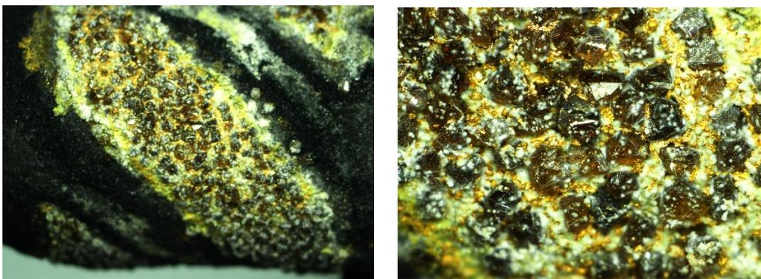
Figure 33: 5% Titanium, 3 days furnace Cooling, Argon as Flushing Gas
