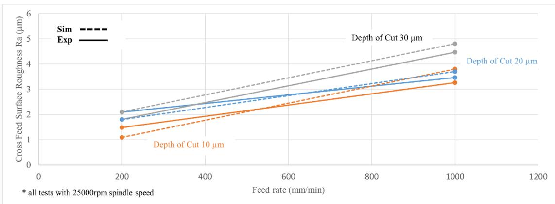
Figure 38: Surface roughness simulation and experimental values for non patterned Wheel
