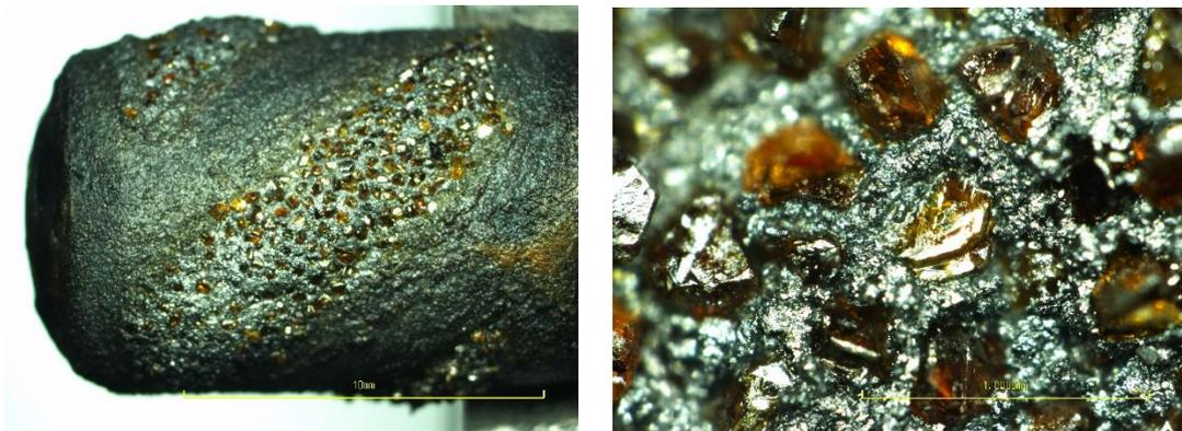
Figure 32: 5% Titanium, Air Cooling, Carbon Dioxide as Flushing Gas
