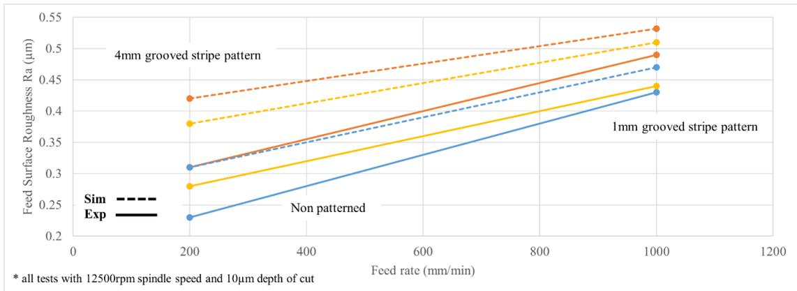
Figure 39: Surface roughness simulation and experimental values for non patterned Wheel comparing to stripe patterned
