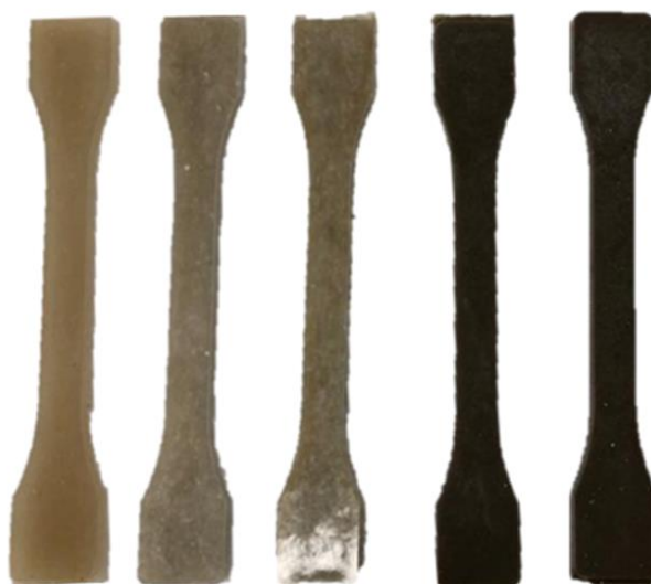
Figure 13 Injection molded samples from left to right 10WC, 20WC, 30WC, 20WC10VC, and 10WC10VC.
