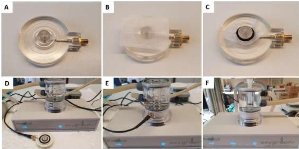
**Figure 8. Components of Clark-type oxygraph and its assembly.** A) a platinum electrode; B) a cigarette paper and a membrane was inserted on top of the electrode; C) paper and membrane are fixed to the electrode with a rubber; D) the electrode connected to device with a cable; E) the electrode connected to the chambers; F) cell solution is put to the chamber for measuring OCR.
