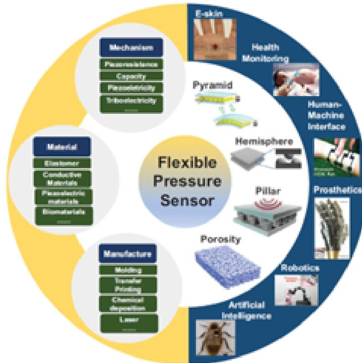
Regarding the material choice of the sensor, as it is earlier stated, it is interrelated to the other two design criteria, i.e. the mechanism and geometry. Earlier well known examples of PR pressure sensors are silicon-based MEMS sensors. Although still often preferred for planar applications, due to their brittle nature, Silicon is not widely used in flexible sensor applications (Chen et al., 2008).
