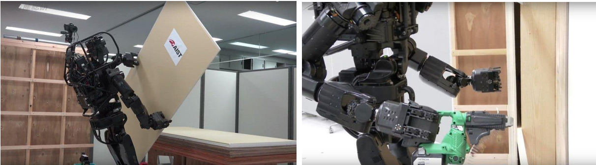
Figure 2.7 HRP-5P Performing Assembly Task without Human Assistance (Kaneko, 2019).
