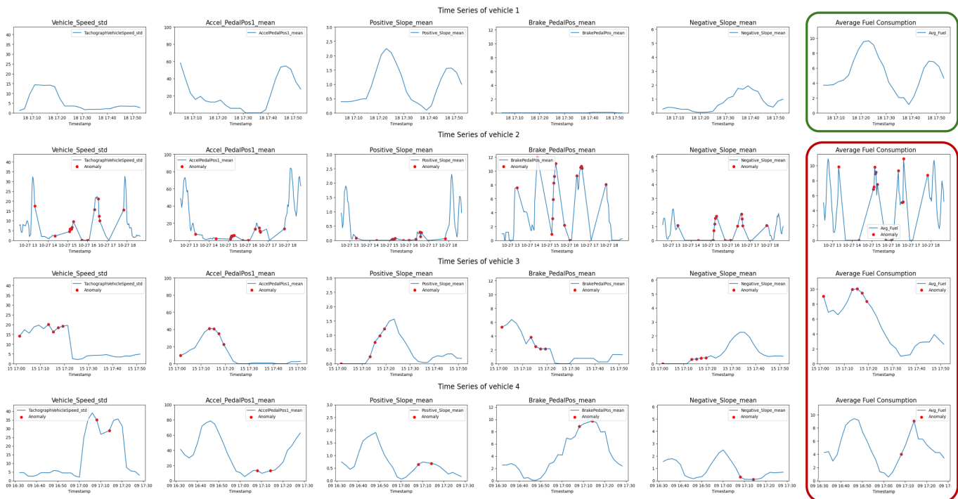
Fig. 3: Time series plots of driving signals and average fuel consumption from sample healthy and anomalous drive cycles of HDVs
