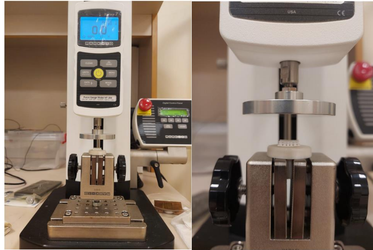
Figure 15. Test setup used for tensile and compression testing using a) MARK-10 UTM machine with b) images during compression testing of scaffolds.
