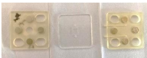
Figure 2 : Magnet holder cartridge system parts in order from left to right: Magnet closure; PDMS mat; Magnet pad
