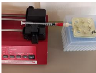
Figure 1: Top view of microfluidic cartridge system
