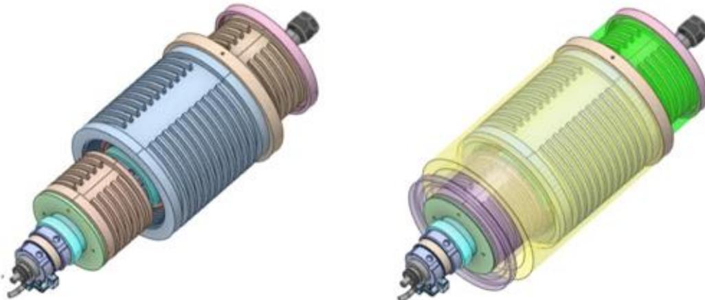
Fig. 3.40 Parallel cooling channel designs
