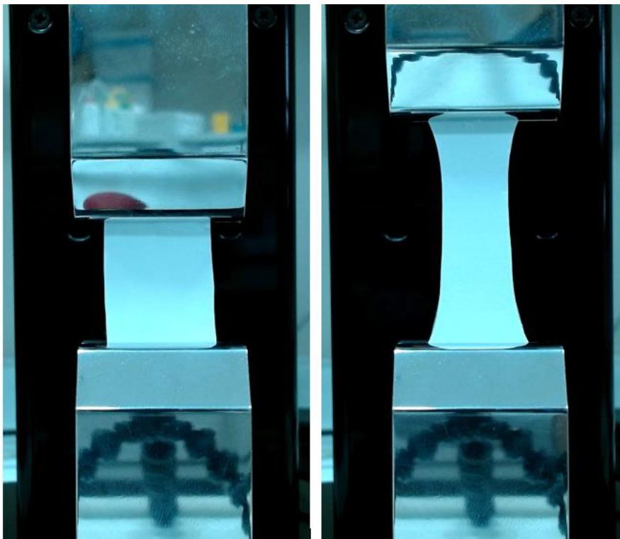
Figure 14 Mechanical test images of PS1 after 1 sec and 50 sec.
