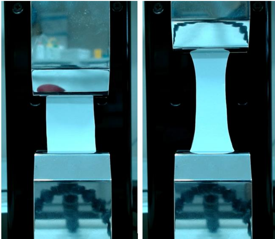
Figure 15 Mechanical test images of PS2 after 1 sec and 50 sec.
