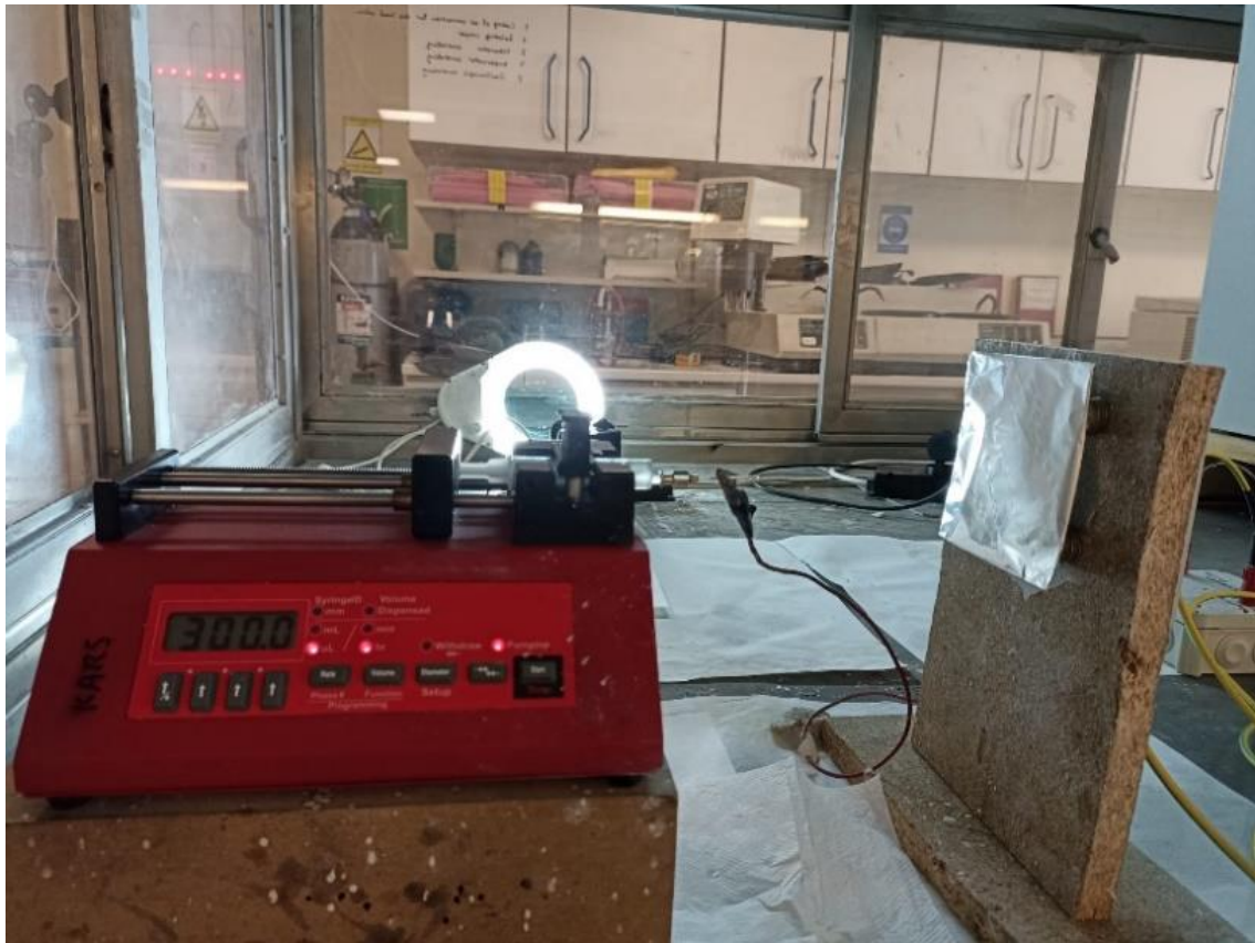
Figure 6 Electrospinning set-up used to produce nanofibers.
