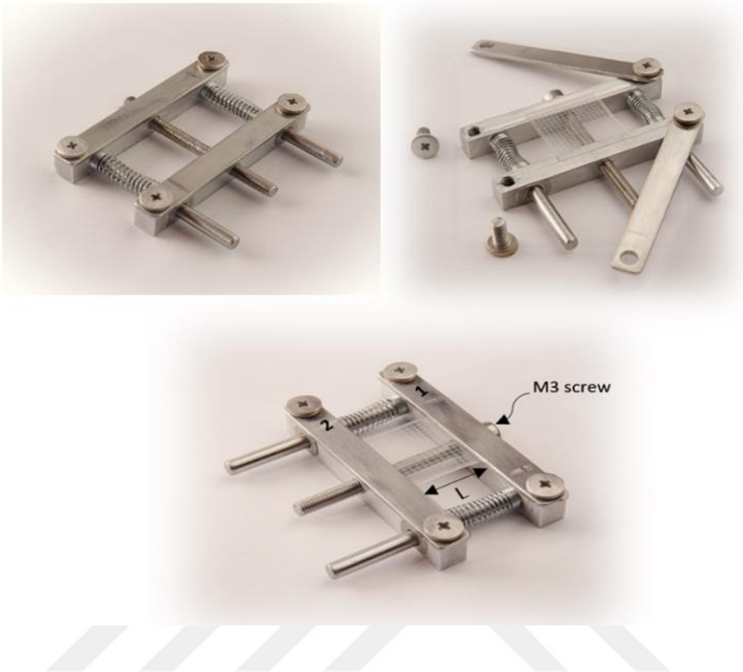
Figure 26: Mounted PDMS on a fabricated stretching apparatus. The sample's initial length before stretching is indicated by the letter L. Bar 1 is fixed and bar 2 moves as the M3 screw rod is turned to stretch the PDMS film.
