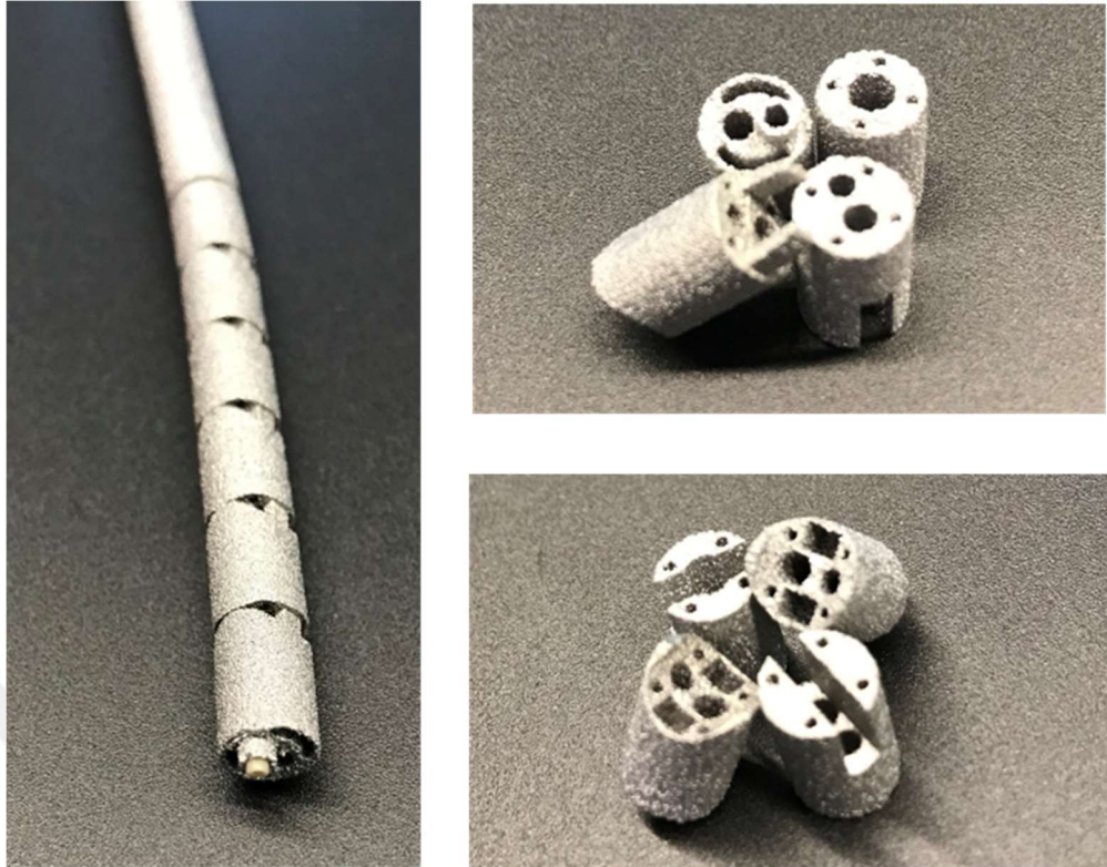
Figure 10 DMLS 3D printed parts with AlSi10Mg material, subfigure in the left shows the assembled cystoscopy probe with metal parts, subfigure in the up-right represents the top view of the small segments of the probe, subfigure in the bottom-right represents the bottom view of the small segments of the probe
