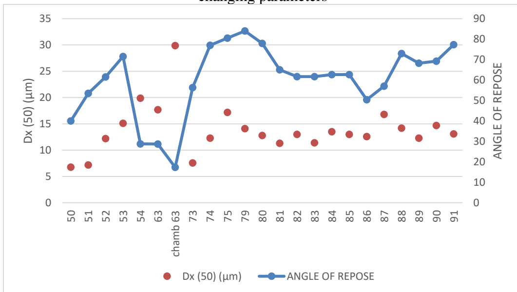
Figure 55. Particle size analysis and flowability resistance relation in the perspective of changing parameters
