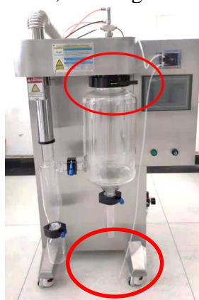
Figure 25. Spray dryer Tefic TFS-2L, showing collecting promising sample position.
