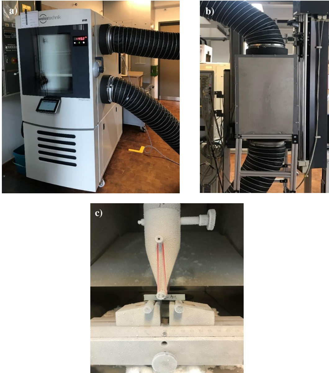
Figure 16: Test set up for -40 °C. a) Cooling machine which has two hoses, upper and lower. b) Upper and lower hoses are connected to the test chamber. c) SENB test configuration with the specimen.
