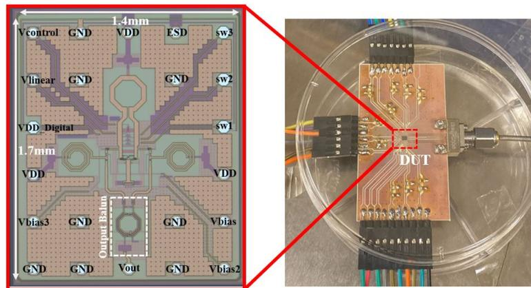
Figure 4.2 Flip-chip assembled Device Under Test
