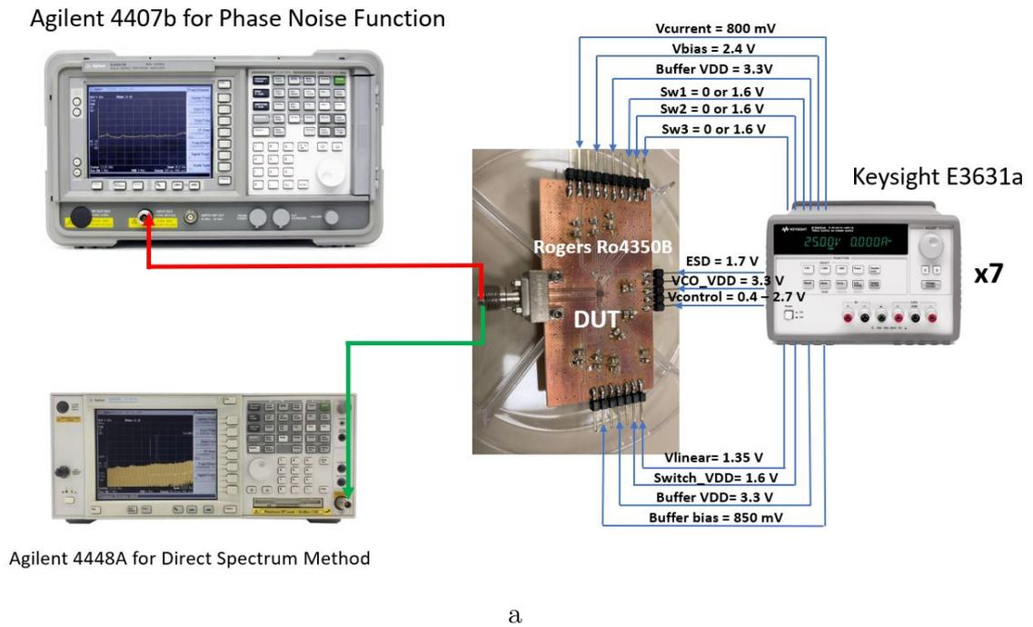
Figure 4.1 VCO Measurement Setup with Agilent 4407b and Agilent 4448A Spectrum Analyzers
