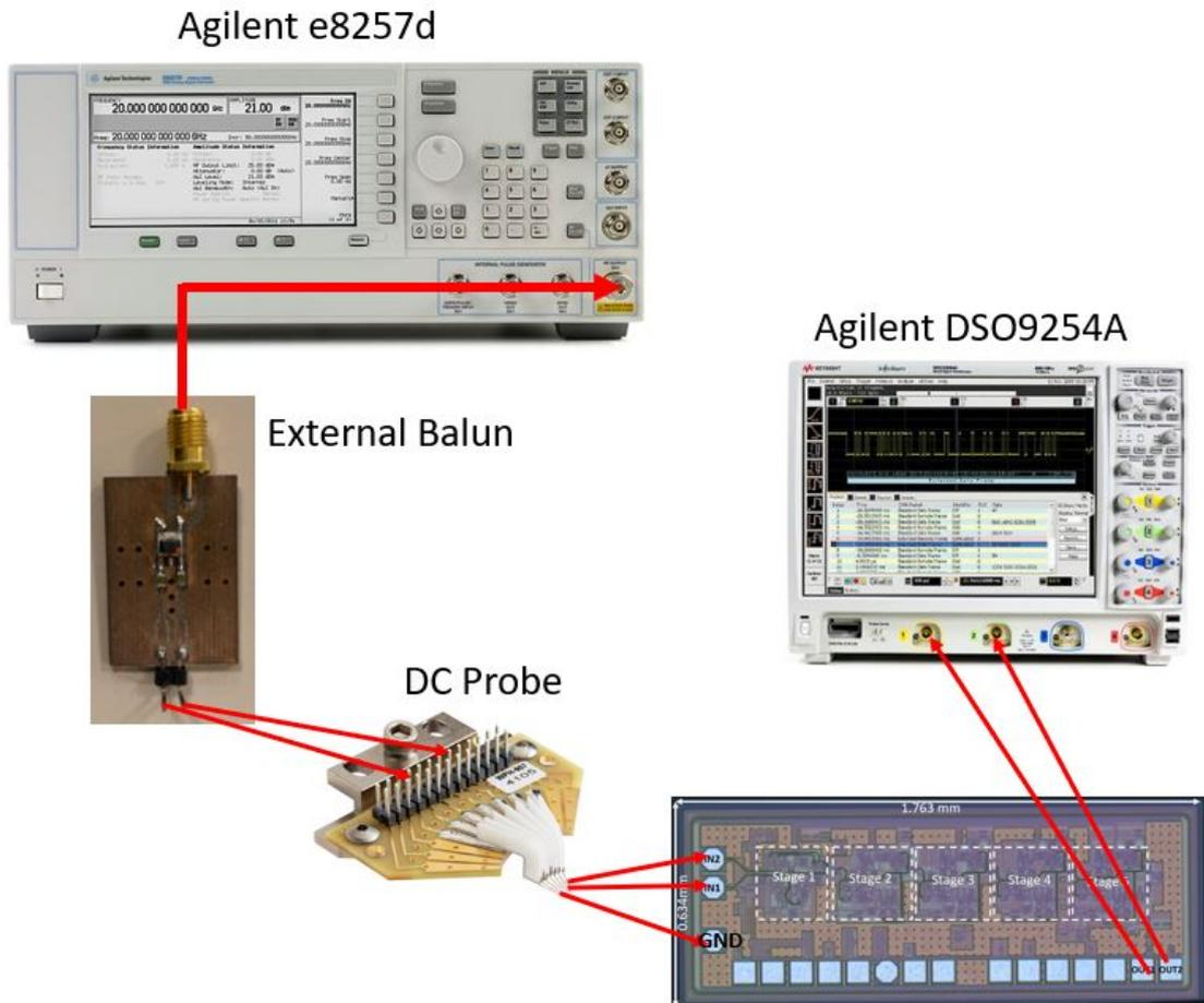
Figure 4.14 Divider Measurement Setup
