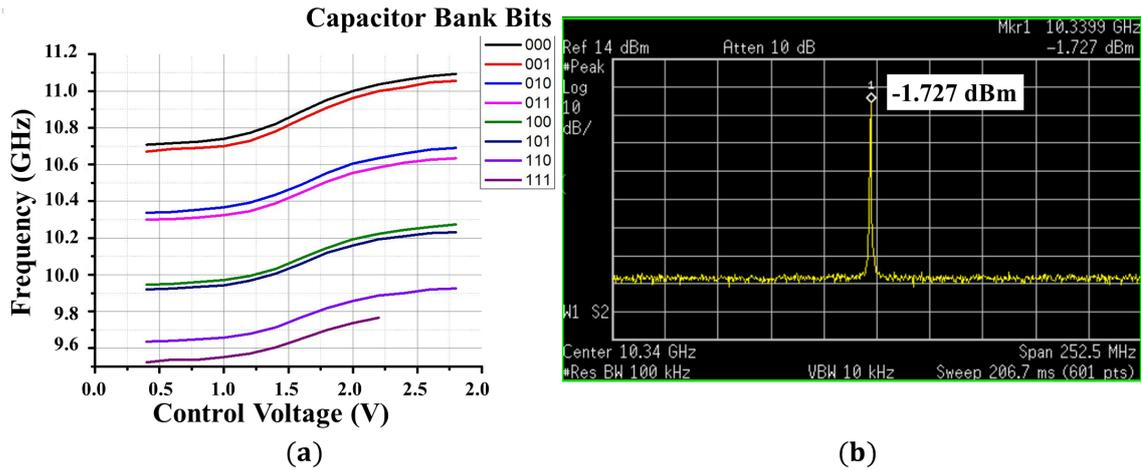
Figure 4.9 a) Frequency Tuning Curves
