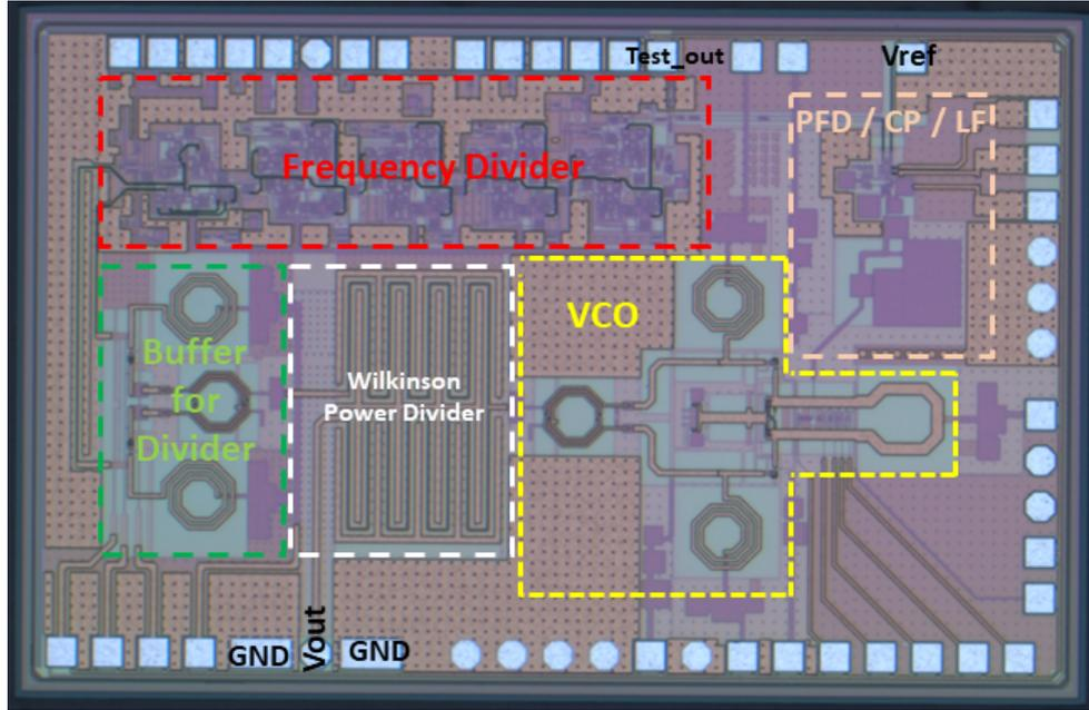
Figure 3.41 Realized Closed Loop PLL Chip
