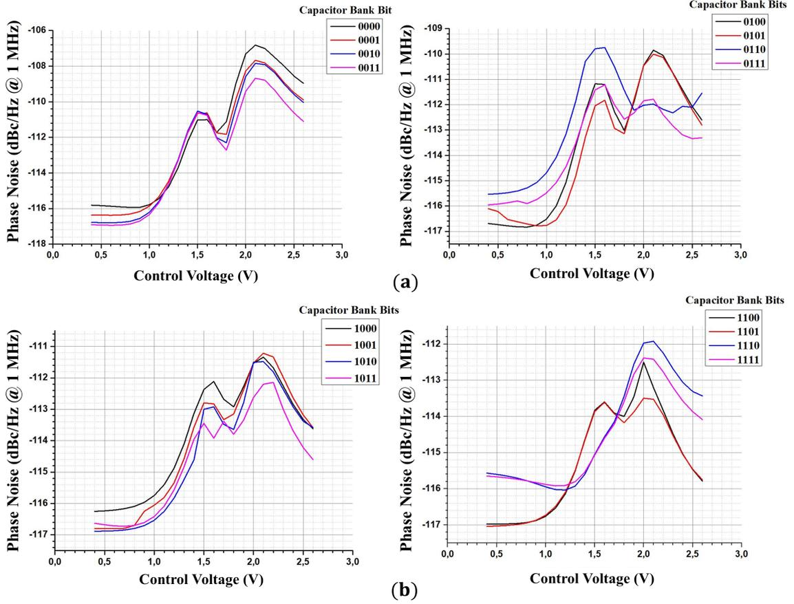
Figure 3.24 PN vs. Control Voltage a) First 8 states b) Last 8 States
