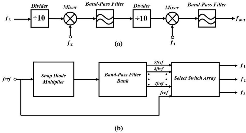
Figure 1.5 Direct Analog Synthesizer Block Diagram
