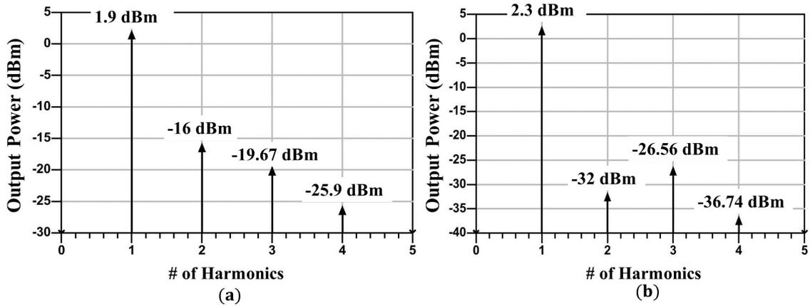
Figure 3.15 Output Spectrum a) W/o Balun b) With Balun
