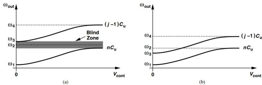
Figure 2.10 a) Frequency Tuning Curves with Blind Zone b) Proper Implementation of Discrete Tuning (Razavi,2011)
