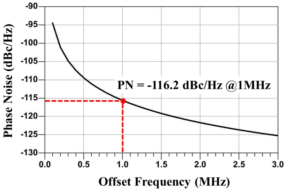
Figure 3.22 PN at Center Frequency
