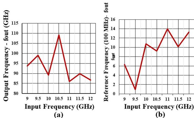
Figure 3.29 a) Output frequency Behaviour with Different Input Frequencies b) Absolute difference between reference and divider output
