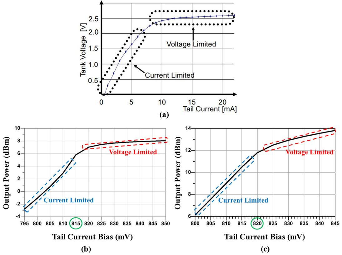
Figure 3.2 (a) Example of Current and Voltage Limited Regions
