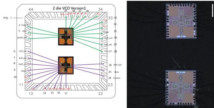
Figure 4.12 The bonding diagram for the VCO and its realization on a 44pin Chip Carrier
