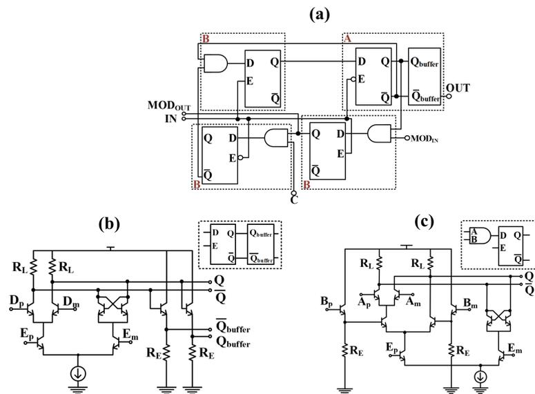
Figure 3.26 a) Block Diagram of 2/3 Cell b) D-latch with buffers c) D-latch with AND gate
