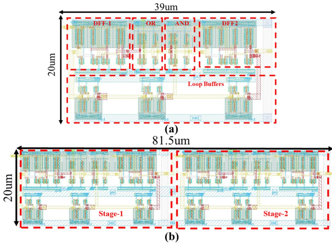
Figure 3.33 a) Single Stage b) Two Stage CMOS Divider Cell Layout
