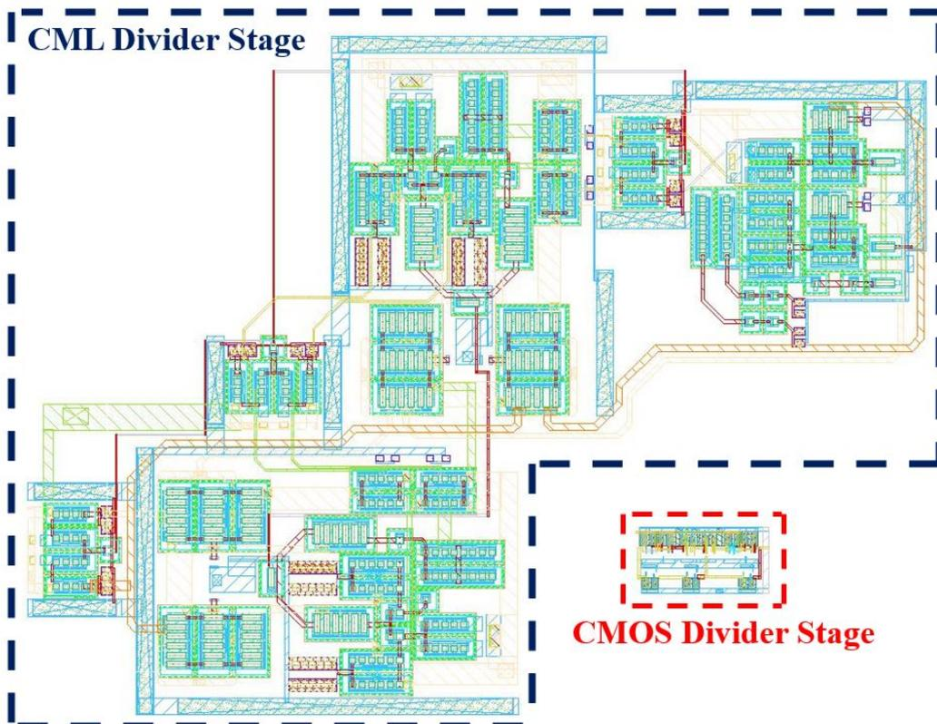
Figure 3.34 Area Comparison of Single CML and CMOS 2/3 Cells
