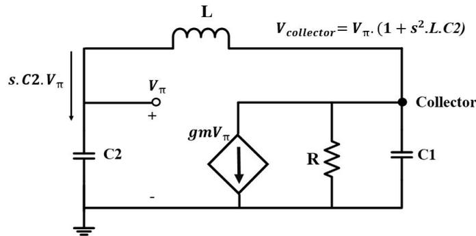
Figure 2.5 Colpitts Oscillator Small Signal Model
