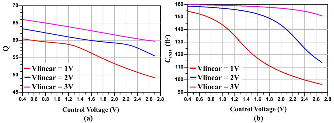
Figure 3.10 Effect of Different  $V_{linear}$  Voltages on a) Quality Factor b) Change of Capacitance
