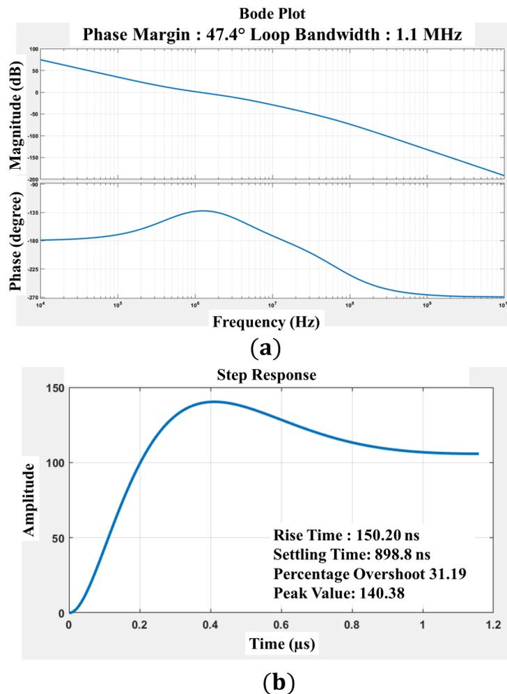
Figure 3.43 Simulation of a) Bode plot of Open-Loop System b) Step Response of the Closed Loop
