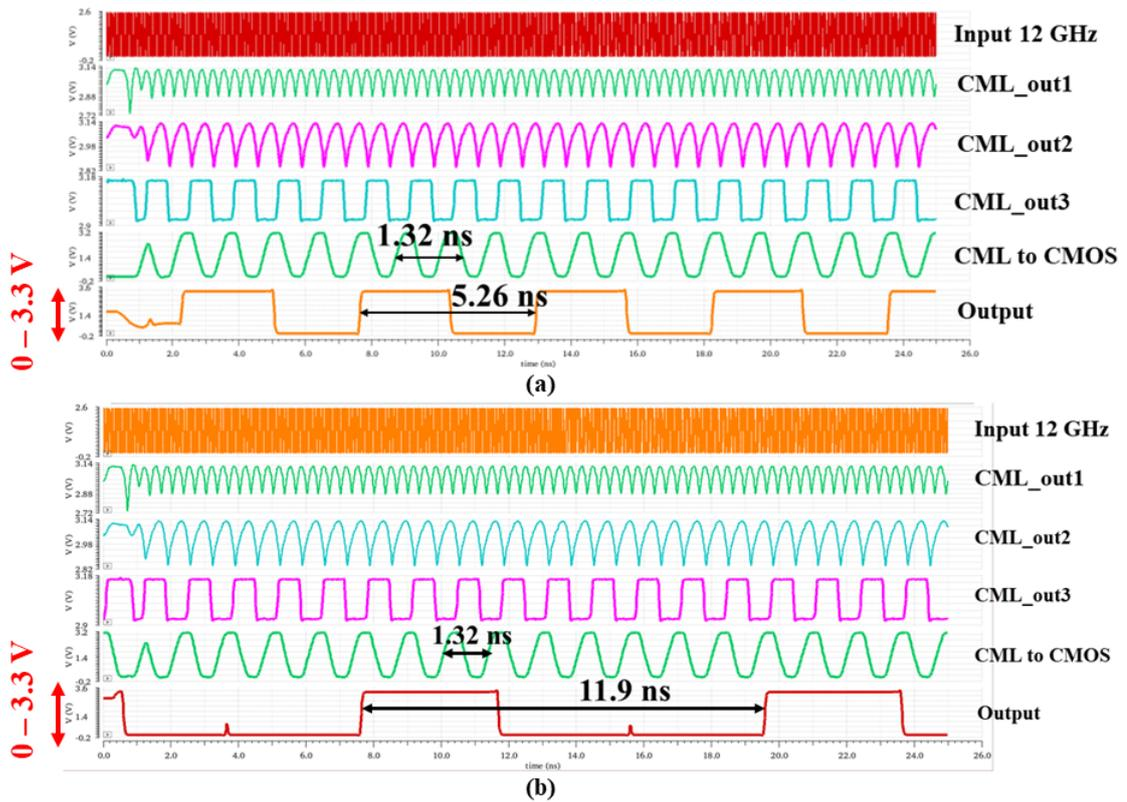
Figure 3.36 Complete Simulation Results of the Designed Divider CMOS Divider Stages Perform Divide by a) Four b) Nine
