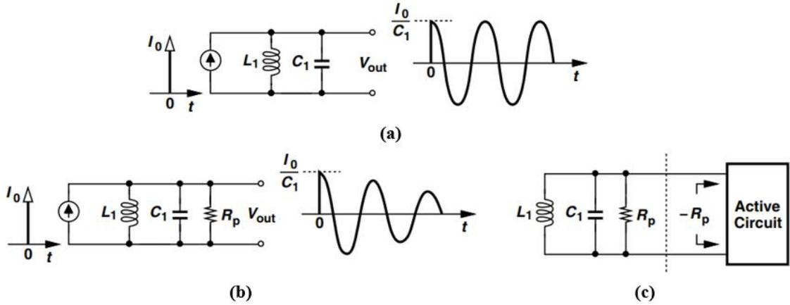
Figure 2.3 a) Response of an Ideal Tank to an Impulse b) Tank circuit with Loss c) Removing of the loss with negative resistance
