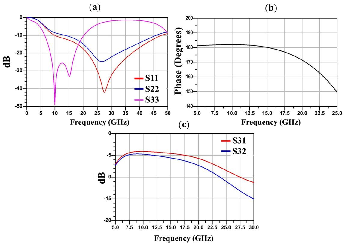
Figure 3.16 a) Input Matching b) Phase c) Loss of the Designed Output Balun
