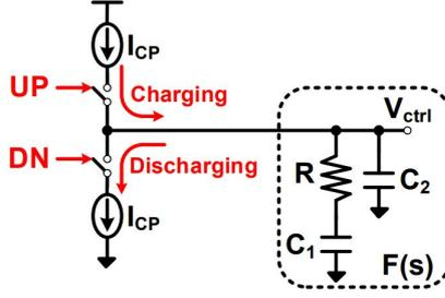
Figure 2.14 Charge Pump Operation with Loop Filter
