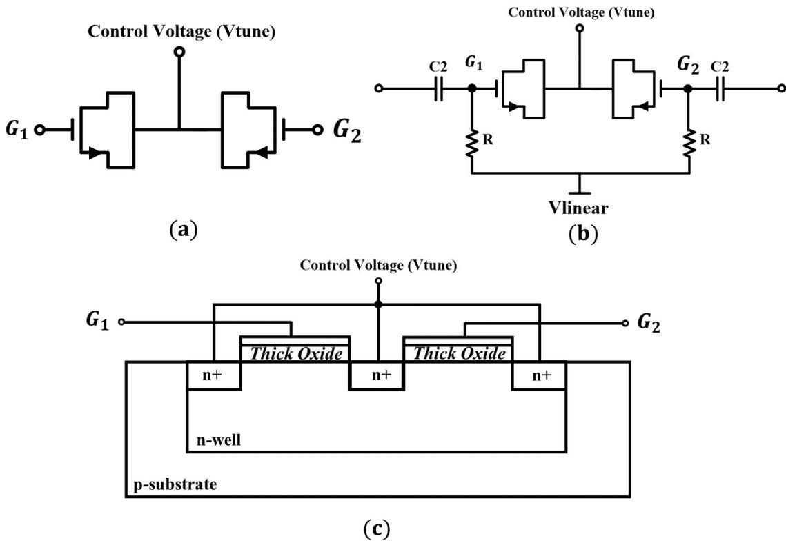
Figure 3.8 a) Basic Varactor Design b) Linearity Control Voltage  $V_{\text{linear}}$  Connection c) Varactor Cross-section
