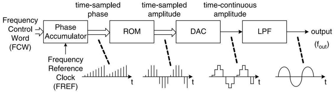
Figure 1.6 Direct Digital Synthesizer Block Diagram (Stazewski & Balsara, 2006)
