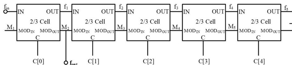
Figure 3.25 Block Diagram of the Initial Design with five 2/3 cells
