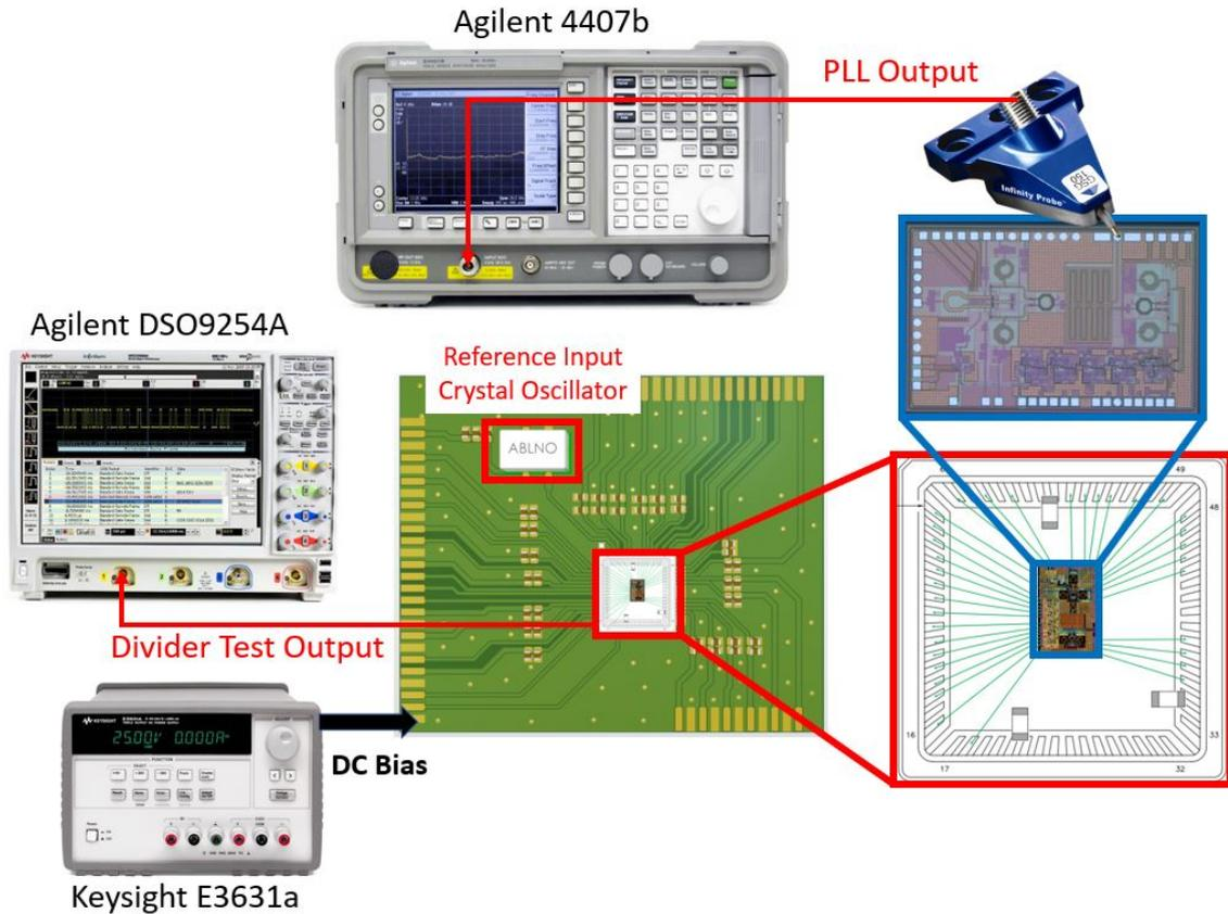
Figure 4.16 Closed Loop Measurement Setup
