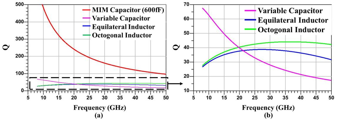
Figure 3.5 Quality Factor Comparison of Tank Components in the technology
