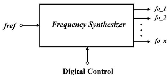
Figure 1.4 Basic Frequency Synthesizer Representation
