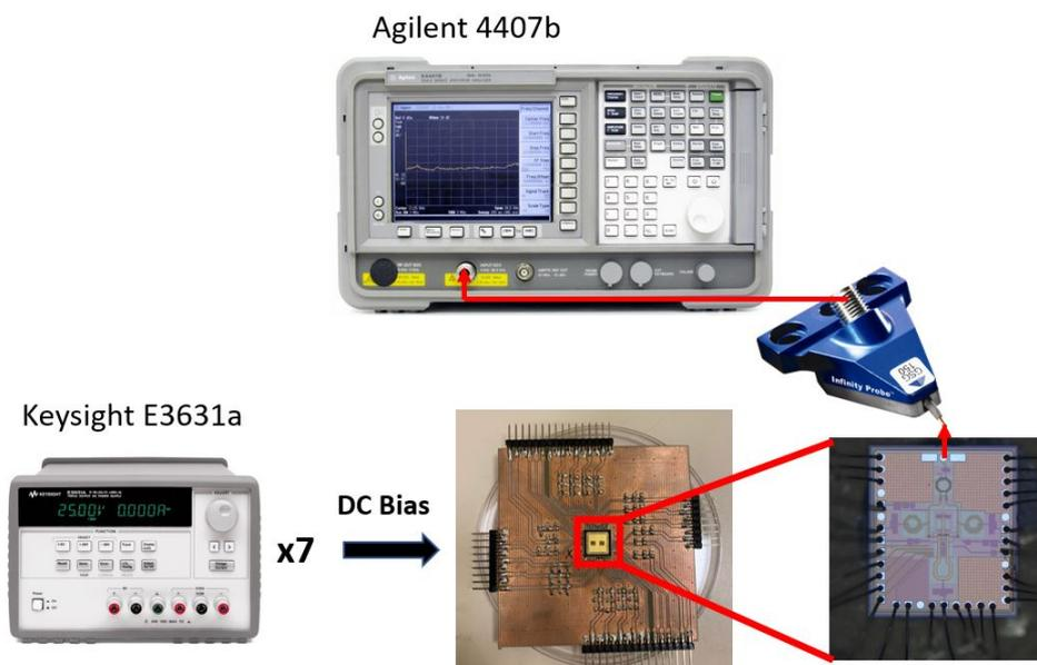
Figure 4.13 The Measurement Setup For the 4-bit VCO
