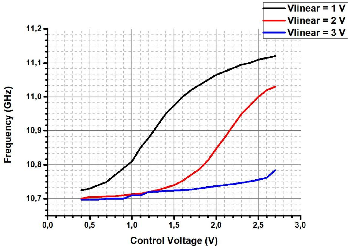
Figure 3.11 Linearity Control Measurement Results
