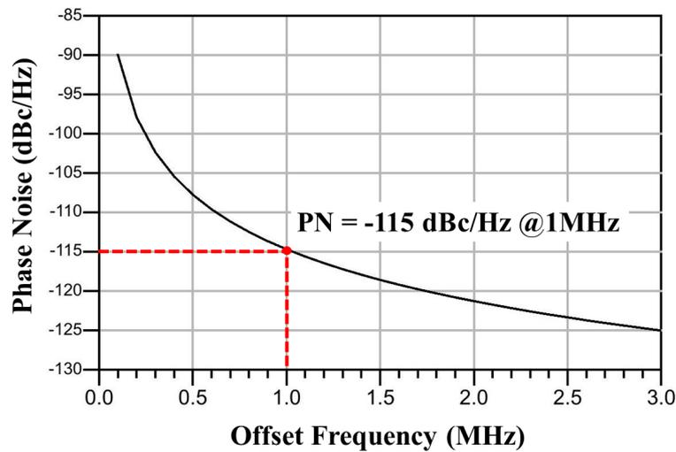
Figure 3.18 PN at Center Frequency
