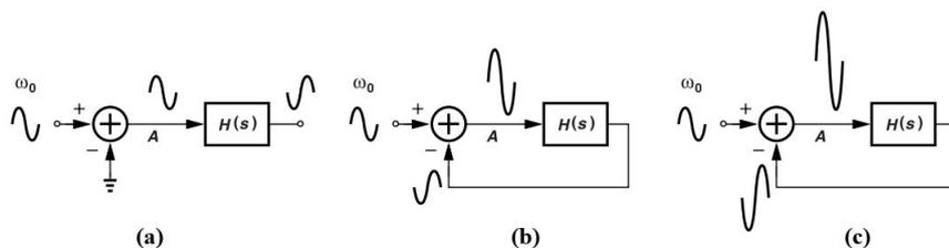
Figure 2.2 Growth of a Oscillation In the feedback due to  $H(jw_0) = -1$  (Razavi,2020)
