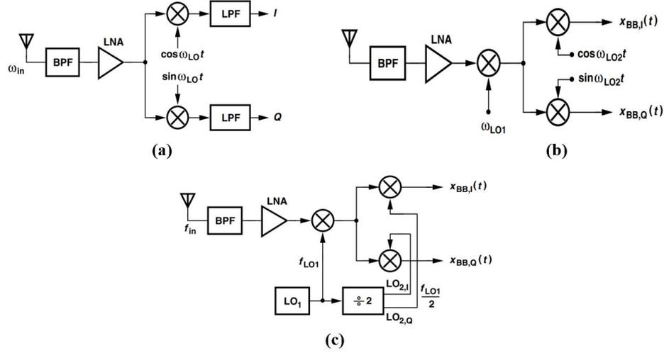
Figure 1.3 Different Frequency Conversion Techniques Used in Receivers (a) Direct (b)Heterodyne (c) Sliding-IF based
