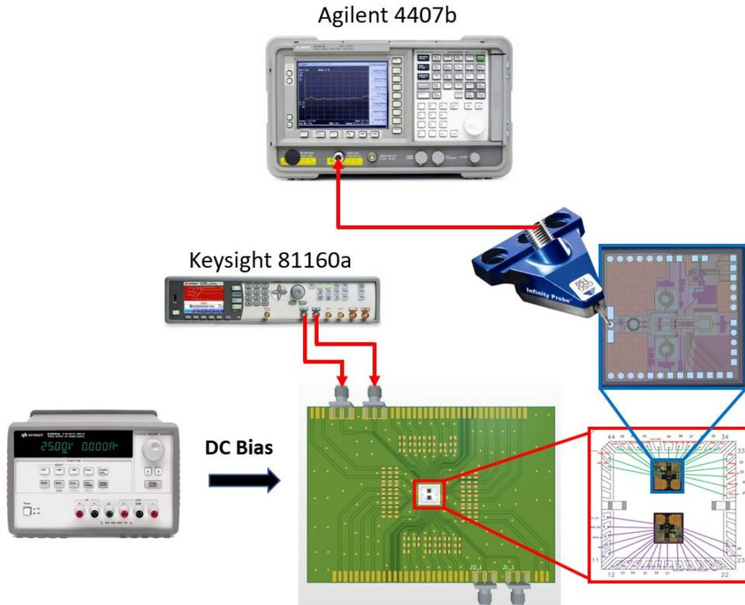
Figure 4.15 Open Loop Measurement Setup
