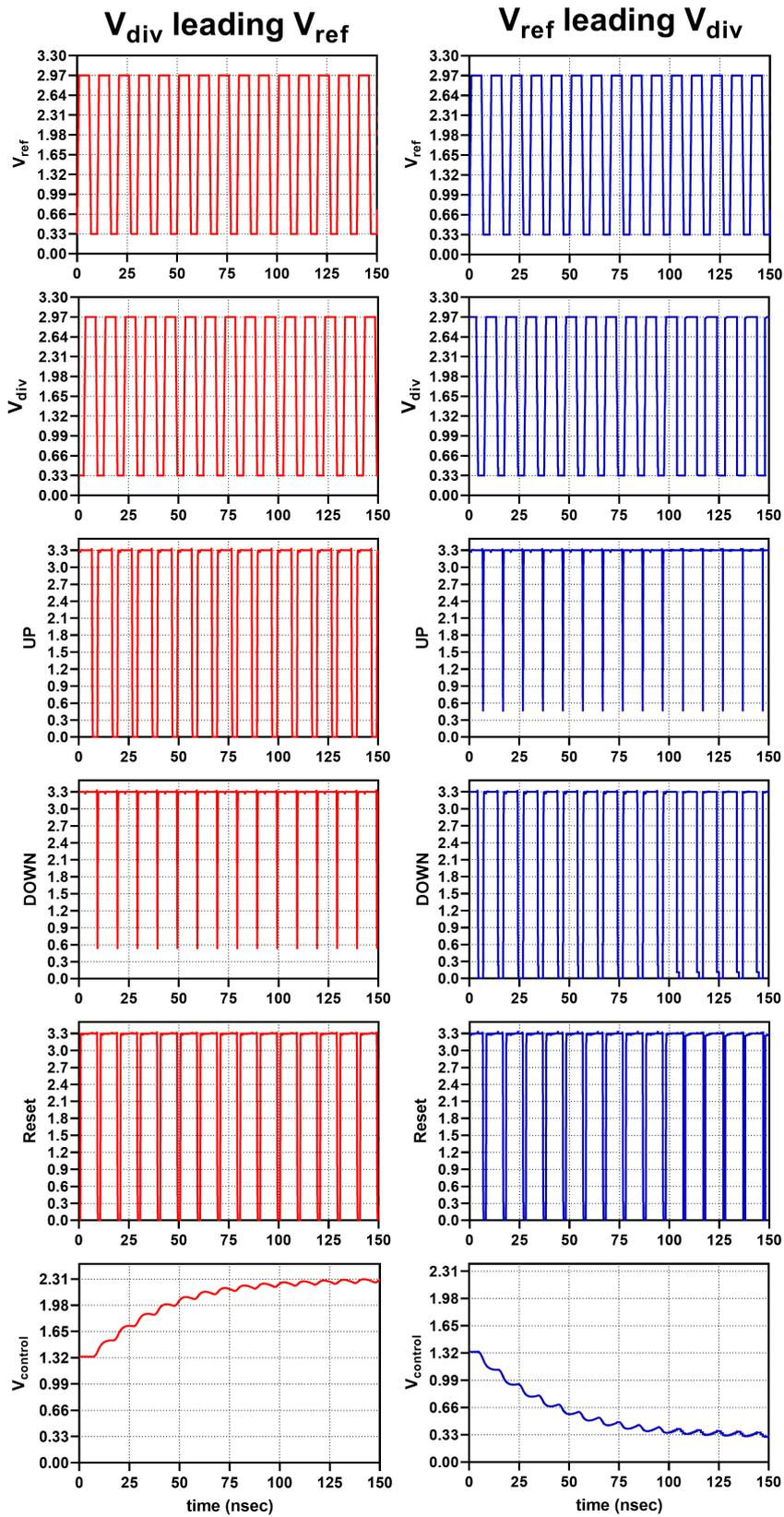
Figure 3.39 Simulation Results of PFD accompanied with CP and LF
