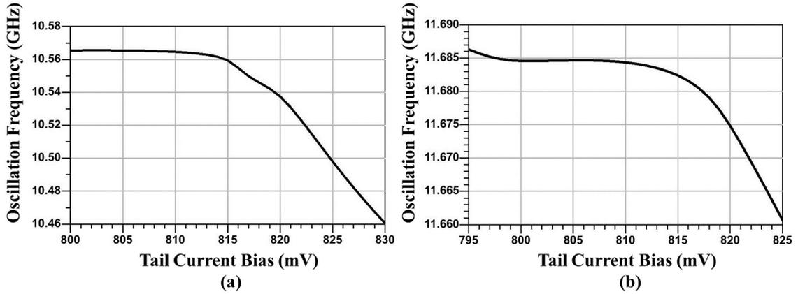
Figure 3.3 Change of Frequency with Tail Current
