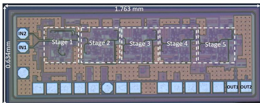
Figure 3.27 Micrograph of The Fabricated Divider
