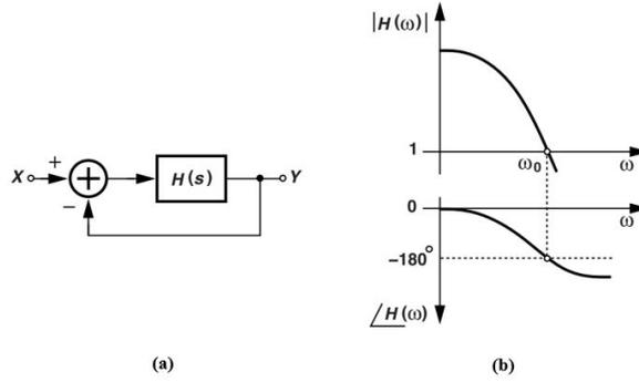
Figure 2.1 a) Negative Feedback System b) Open Loop Frequency Response (Zero Phase Margin) (Razavi,2011)
