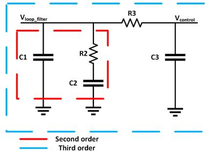
Figure 3.40 Third Order Loop Filter Design For the Synthesizer
