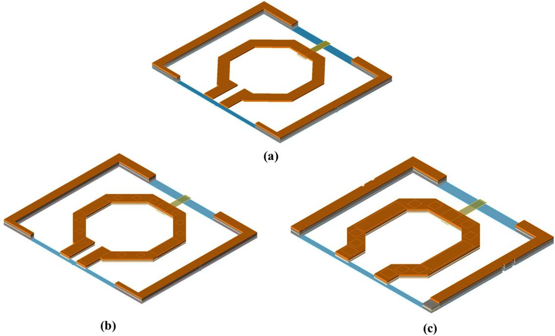
Figure 3.7 3D view of Inductor Designs
