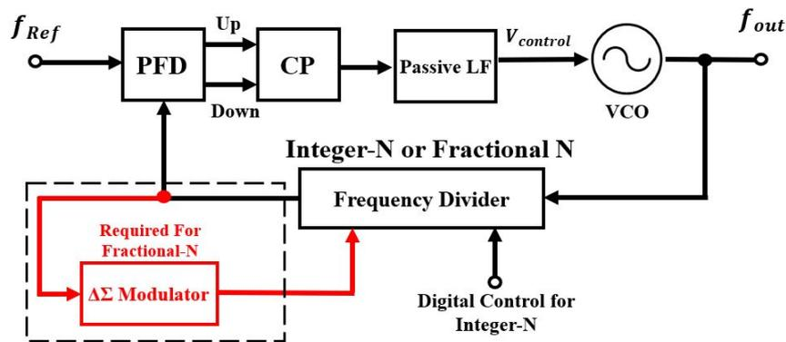
Figure 2.11 Block Diagram of Analog CP PLL
