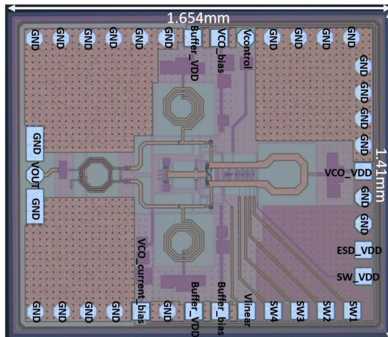
Figure 3.21 Second Version VCO Realized in IHP SG13S Technology for Wire-Bonding and Probe Measurement
