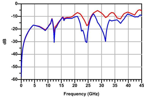
Figure 4.4 Matching of the RF-line on the Test Board
