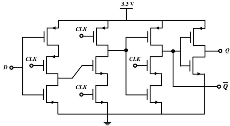
Figure 3.32 TSPC D-Flip Flop
