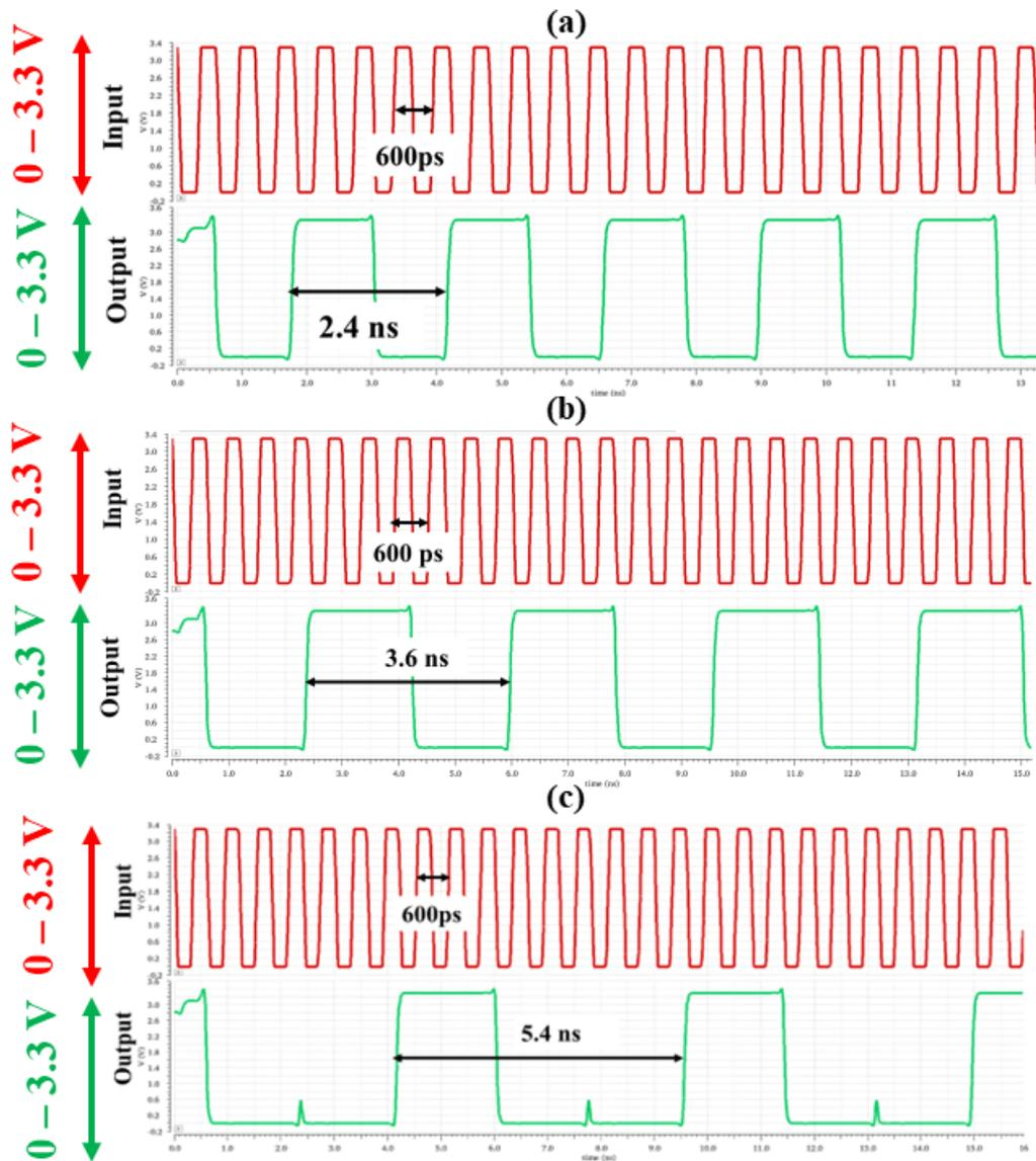
Figure 3.35 2-stage Standalone Simulation Results of the Designed Divider Divide by a) Four b) Six c) Nine
