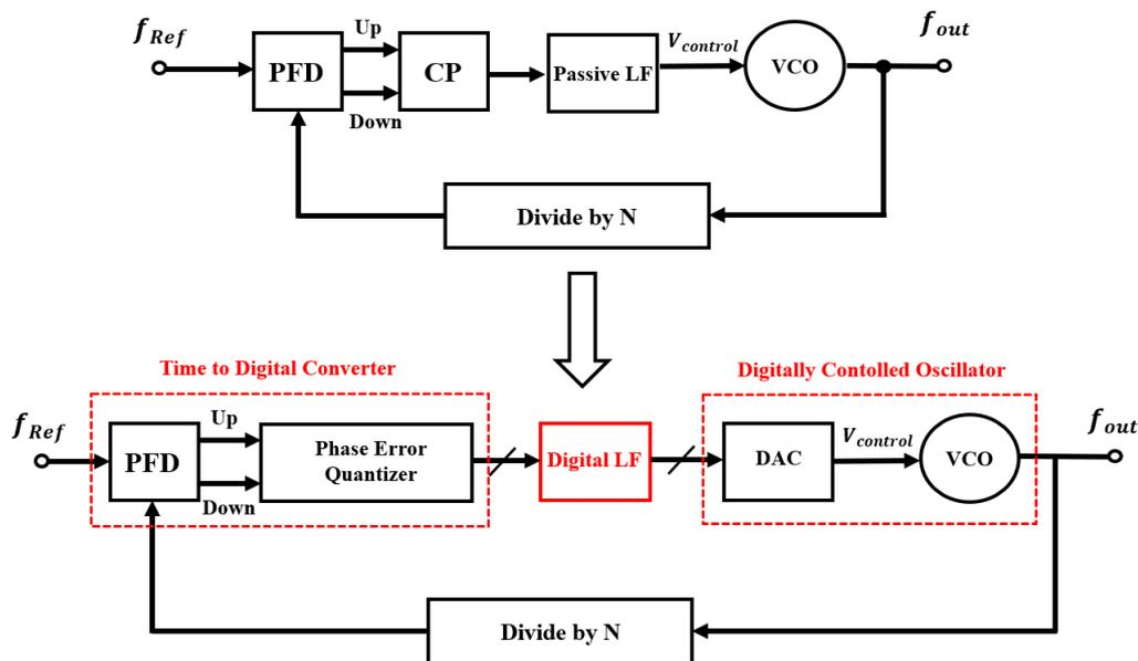
Figure 2.12 Digital PLL Building Block Comparing with the Analog PLL
