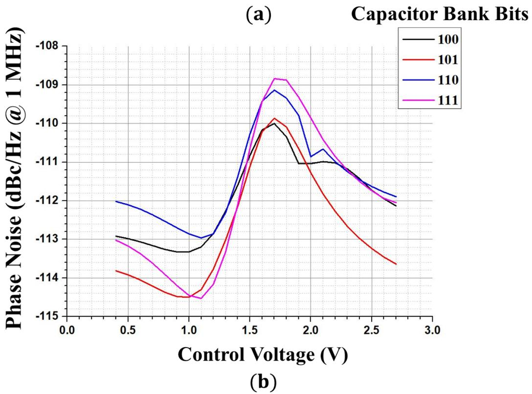
Figure 3.20 PN vs. Control Voltage a) First 4 bit states b) Last bit 4 States
