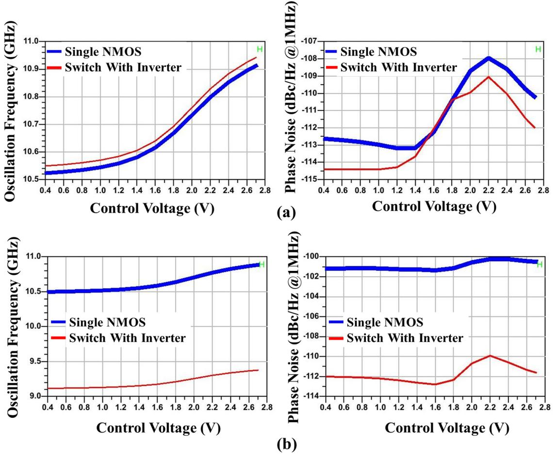
Figure 3.13 Effect of the Inverter at the Bank Switch when All switches are a) Open b) Closed
