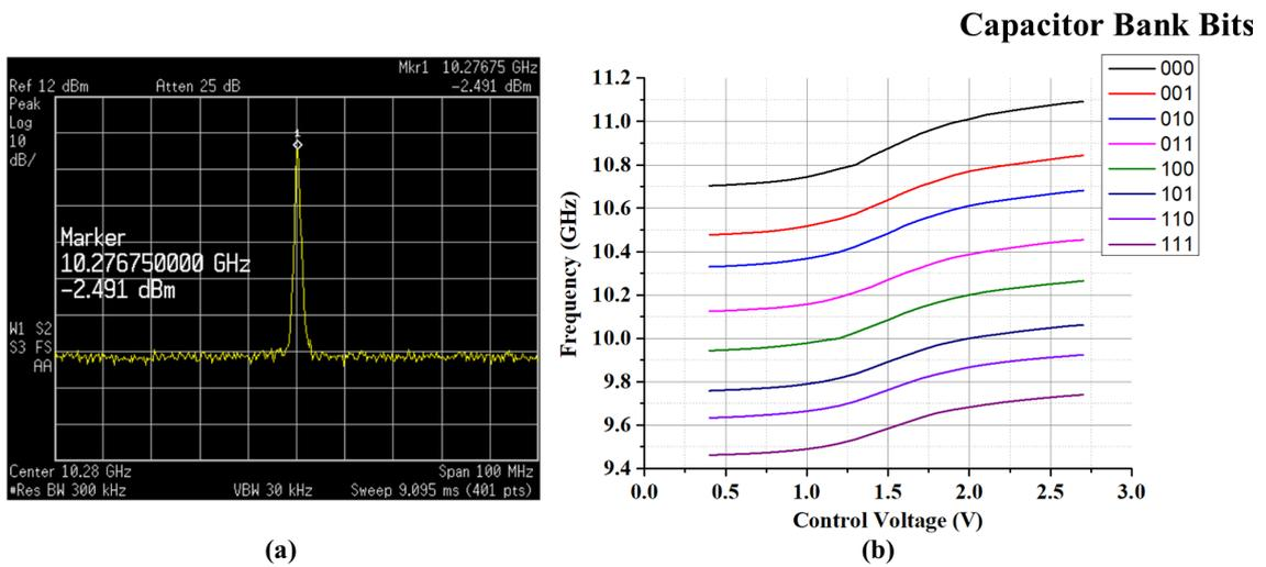
Figure 4.11 a) Spectrum View at Center Freq b) Measured Frequency Tuning Curves
