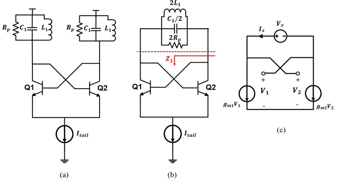
Figure 2.6 a) General CC topology b) Differential Tank Circuit c) CC pair negative impedance calculation
