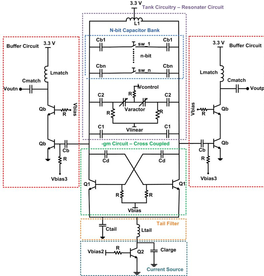
Figure 3.1 Schematic of the Designed VCO
