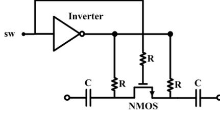
Figure 3.12 Capacitor Bank Switch with Inverter
