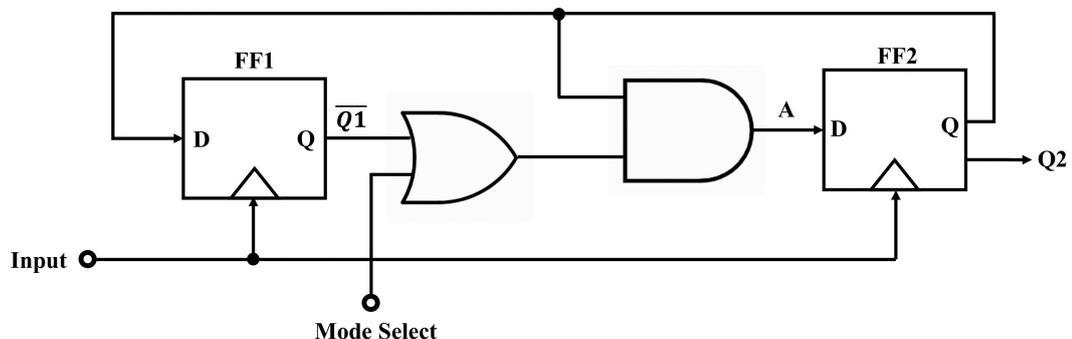
Figure 3.31 CMOS Dual Modulus Design Used for Implementation
