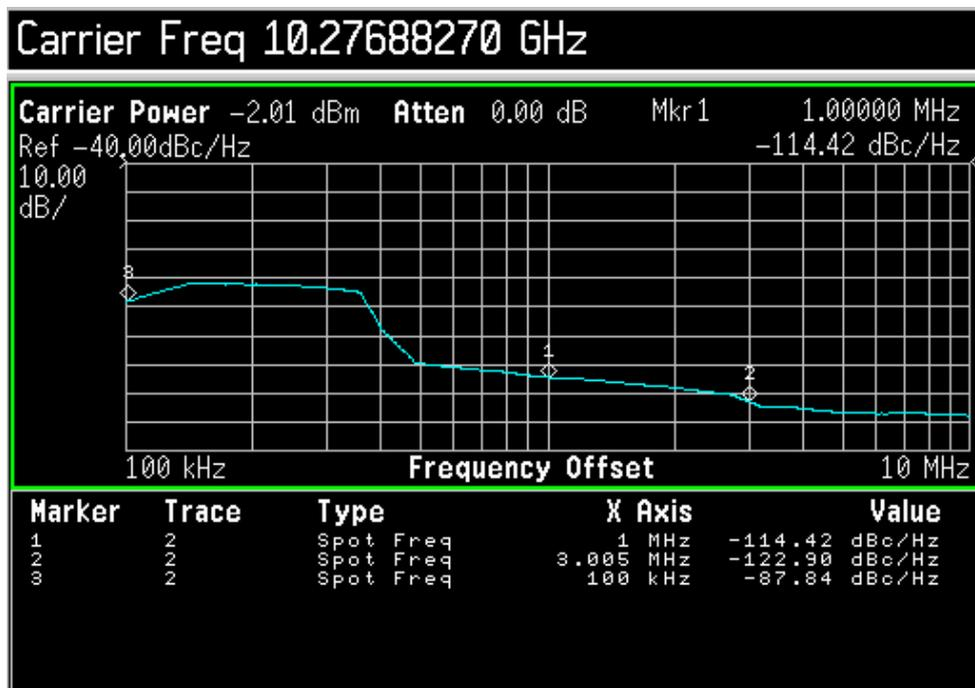
Figure 4.10 PN at Center Frequency
