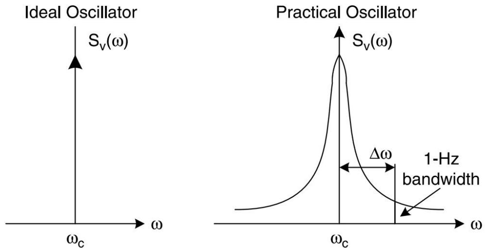
Figure 2.7 The broadening of an impulse due to Phase Noise
