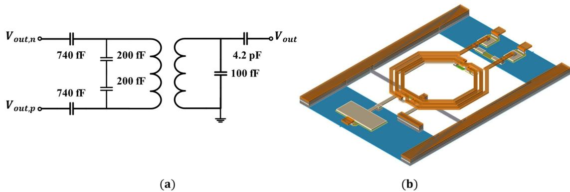
Figure 3.14 a) Schematic View b) 3D layout View of the Output Balun
