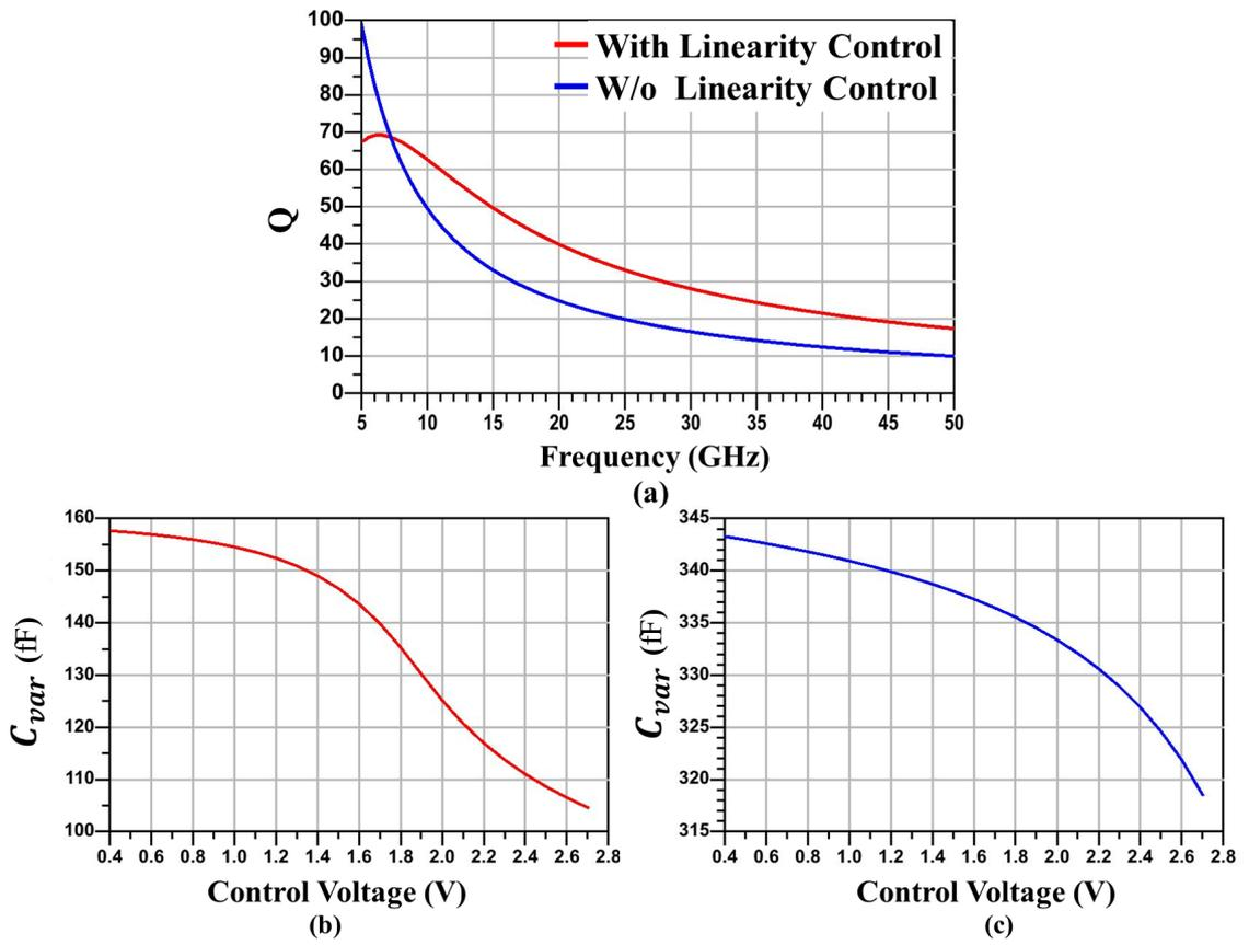
Figure 3.9 a) Effect of the Proposed method on Quality Factor Change of the  $C_{max}/C_{min}$  b) With the Linearity Control, c) W/o the control
