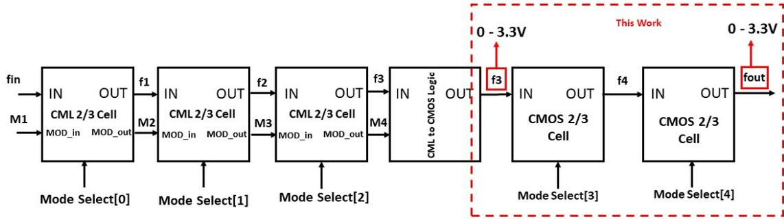
Figure 3.30 Block Diagram of the New Divider
