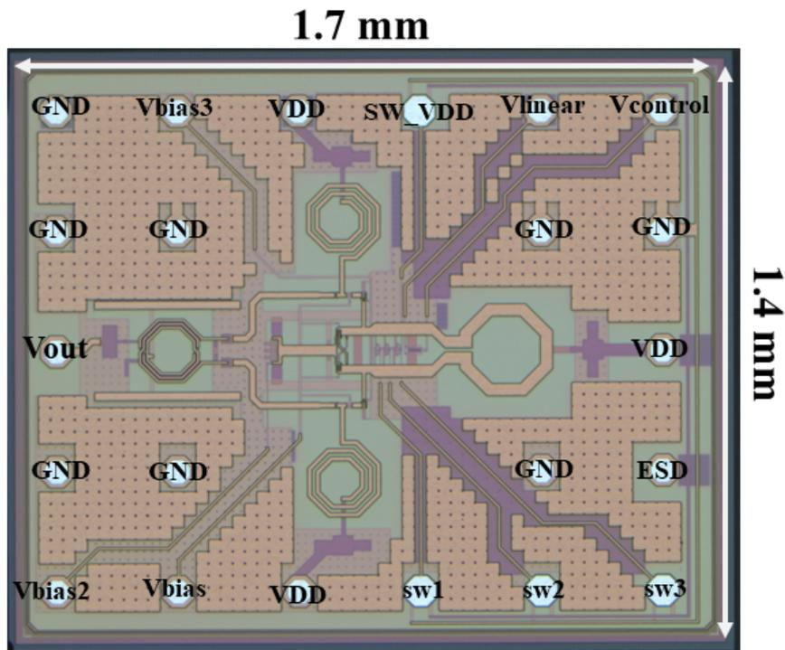
Figure 3.17 3-bit VCO Realized in IHP SG13S Technology for Flip-Chip Assembly
