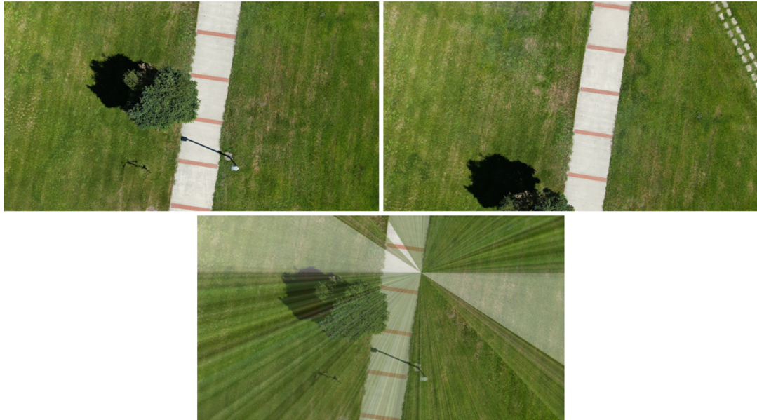
FIGURE 3.21: Fail of Feature-based Stitching Algorithm
