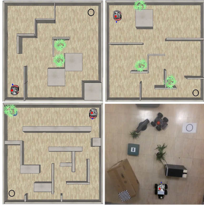
FIGURE 4.10: ArUco Marker Pose Estimation of UGV in All Test Scenes Left Top Image: Scene-1(V-rep), Right Top Image: Scene-2(V-rep), Left Down Image: Scene-3(V-rep), Right Down Image: Scene-4 (Real Setup)
