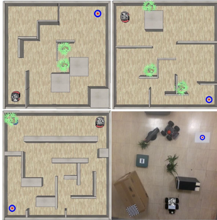
FIGURE 4.11: Circle Detection (Desired Point Detection) Left Top Image: Scene-1(V-rep), Right Top Image: Scene-2(V-rep), Left Down Image: Scene-3(V-rep), Right Down Image: Scene-4 (Real Setup)
