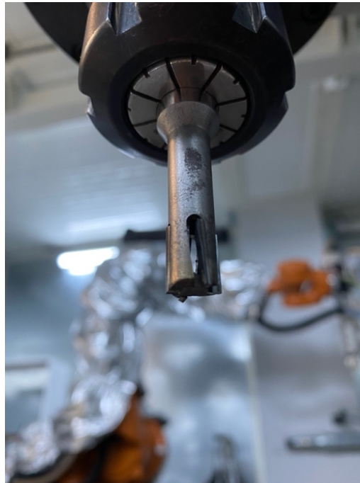
Figure 45: Designed tool with vacuuming gaps
