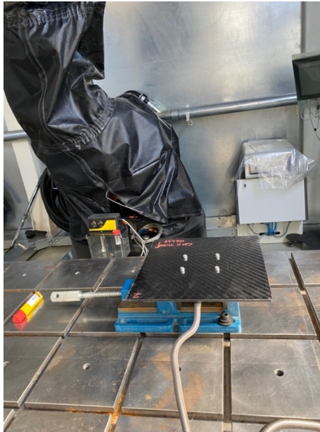
Figure 53: CFRP plate, fixture, and dynamometer
