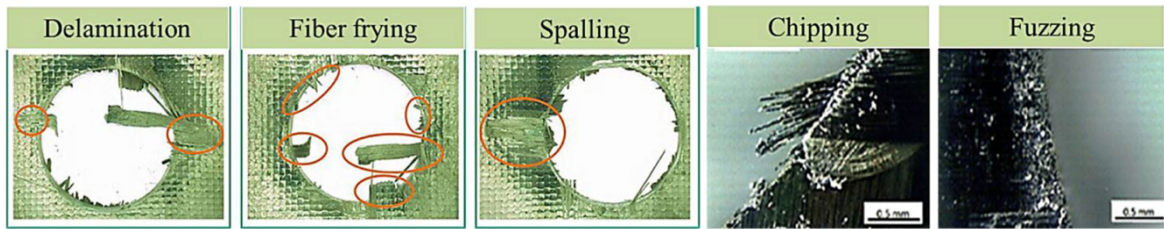
Figure 5: Delamination, fiber frying, spalling, chipping and fuzzing [17]
