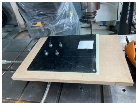
Figure 14: UD CFRP plate attached to glass fiber and MDF layer
