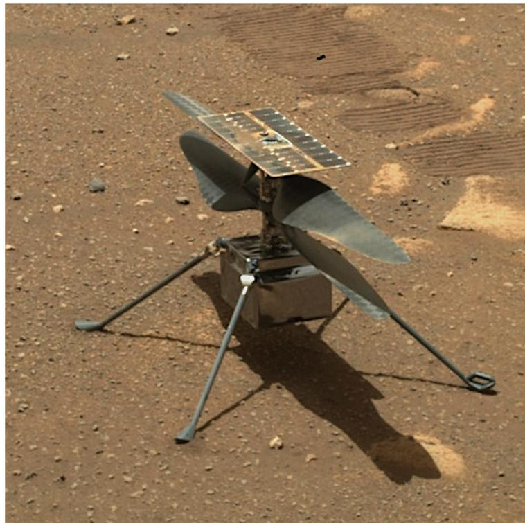
Figure 1.2 Martian helicopter Ingenuity mainly uses COTS parts. Such as a Qualcomm Snapdragon 801 mobile phone SoC for image processing (Tzanetos, Aung, Balaram, Grip, Karras, Canham, Kubiak, Anderson, Merewether, Starch, Pauken, Cappucci, Chase, Golombek, Toupet, Smart, Dawson, Ramirez, Lam, Stern, Chahat, Ravich, Hogg, Pipenberg, Keennon & Williford, 2022).
