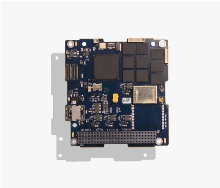
Figure 1.3 AAC Clyde Space’s KRYTEN-M3 satellite on-board computer uses COTS parts and achieves fault-tolerance using a combination of the listed measures (AAC Clyde Space, 2020).
