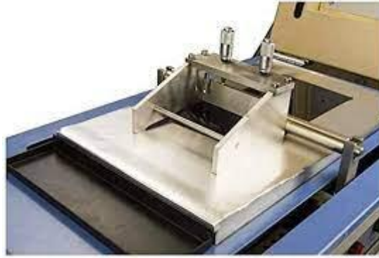
Figure 13 the Dr. blade adjustable film castor/coater. The thickness of film range from 10 microns to 3500 microns.
