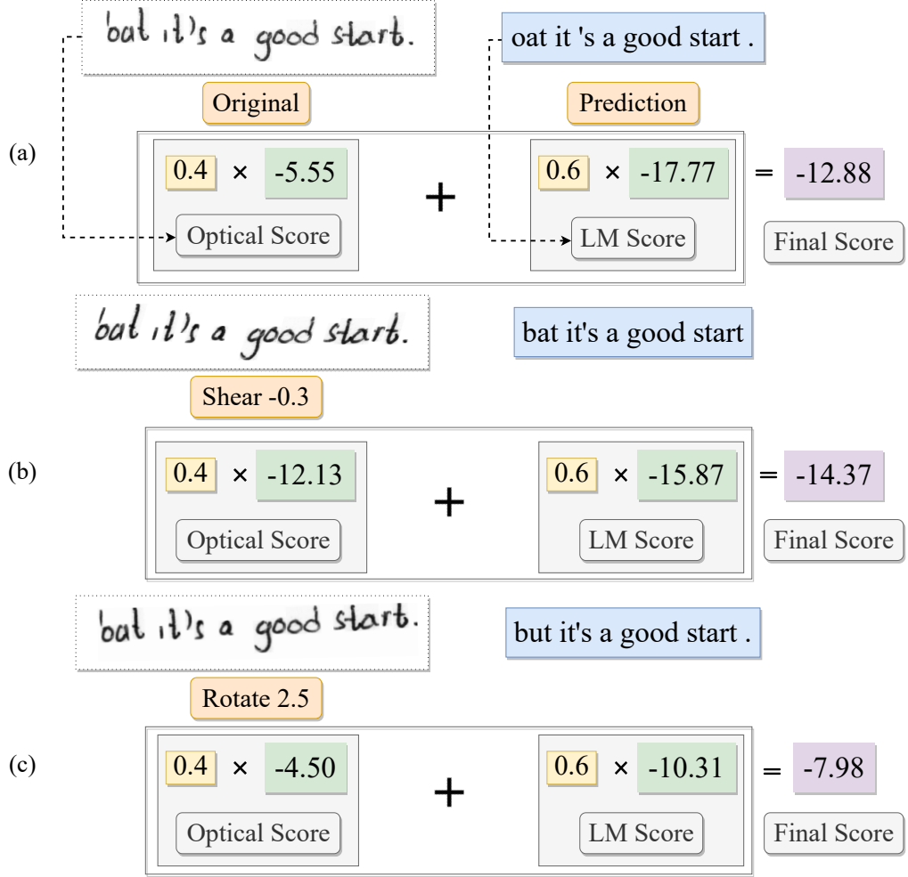
Figure 3.7 An example application of the scoring transcriptions. (a) Output of the original image is scored using the equation 3.1. The optical score is obtained from the deep learning network. The language model score is computed using the 4-gram language model. (b) and (c) shows the scoring steps of the transformed images. The output with the lowest final score is picked as the final output, which is the correct transcription of the handwriting.
