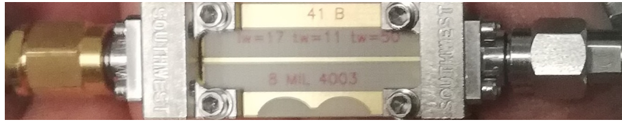
Figure 4.6 IL measurement setup of Southwest end launch connector.
