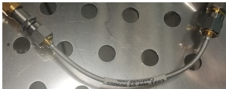
Figure 4.3 IL measurement setup of cables.
