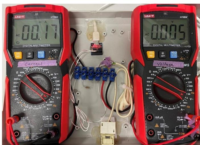
**Figure 35. TEER measurement device designed in the laboratory.** The device composes of a standard USB charger, USB extension cord, and a microcontroller, two standard multimeters to measure alternating current and voltage as root mean square, telephone extension cord with a RJ14 female connector including six pins with the inner four wired, two short cables, a luster terminal, wire and ferrules, and soldering lugs.
