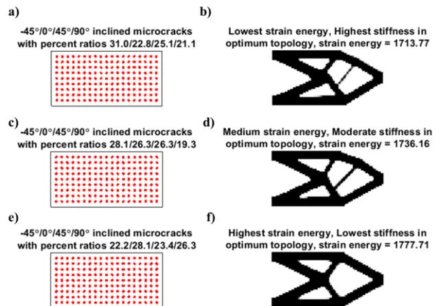
**Fig 6.** Cantilever beam with microcracks ( $L_{crack} = dx/2$ ), a) microcracks orientation for achieving minimum strain energy, b) optimum topology for minimum strain energy, c) microcracks orientation for achieving medium strain energy, d) optimum topology for medium strain energy, e) microcracks orientation for achieving maximum strain energy, f) optimum topology for maximum strain energy.
