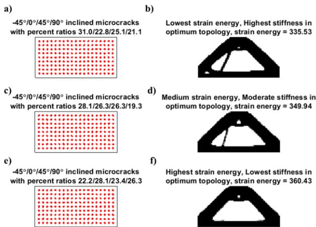
**Fig 7.** Simply supported beam with sets of microcracks ( $L_{crack} = dx$ ), a) microcracks orientation for achieving minimum strain energy, b) optimum topology for minimum strain energy, c) microcracks orientation for achieving medium strain energy, d) optimum topology for medium strain energy, e) microcracks orientation for achieving maximum strain energy, f) optimum topology for maximum strain energy.
