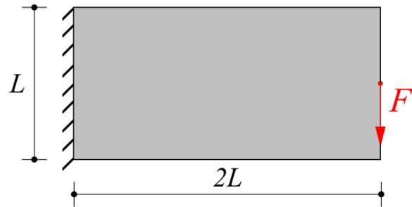
**Fig 5.** Design domain of the cantilever beam.
