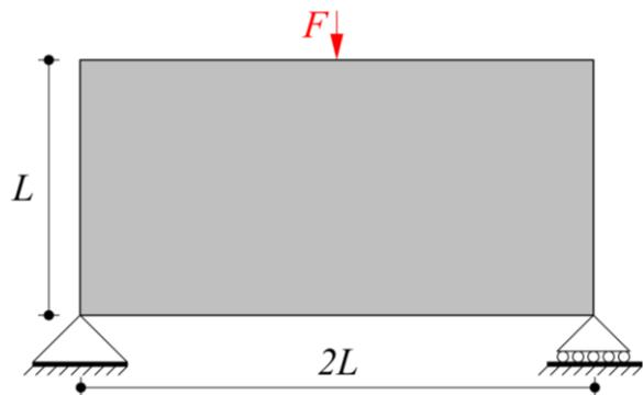
**Fig 3.** Design domain of the simply supported beam.
