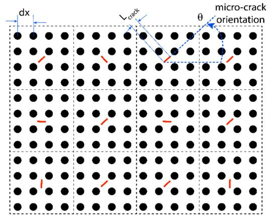
**Fig 2.** Schematic of microcrack in a design domain, black circles represent the particles in PD, the grid of 4 by 4 is located between dashed lines; red lines are microcracks with the size of  $L_{crack}$  and orientation of  $\theta$ .
