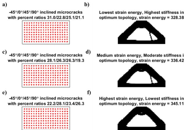
**Fig 4.** A simply supported beam with microcracks ( $L_{crack} = dx/2$ ), a) microcracks orientation for achieving minimum strain energy, b) optimum topology for minimum strain energy, c) microcracks orientation for achieving medium strain energy, d) optimum topology for medium strain energy, e) microcracks orientation for achieving maximum strain energy, f) optimum topology for maximum strain energy.
