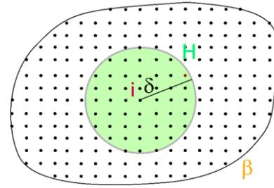
Fig 1. Horizon-Family of the material point  $i$  for PD model.
