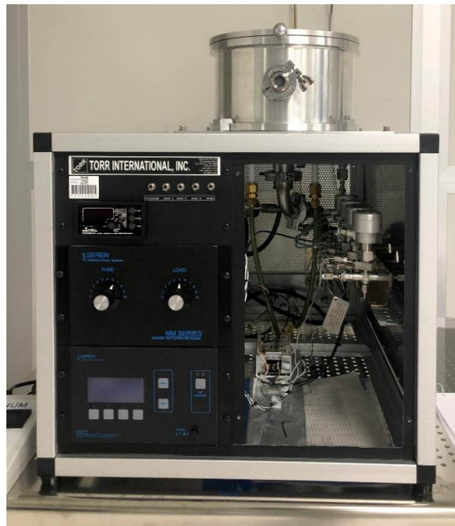
Figure 15 Torr International Oxygen Plasma Asher-R301.
