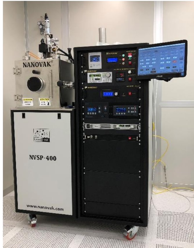
Figure 19 Nanovak ® Sputter NVSP-400.
