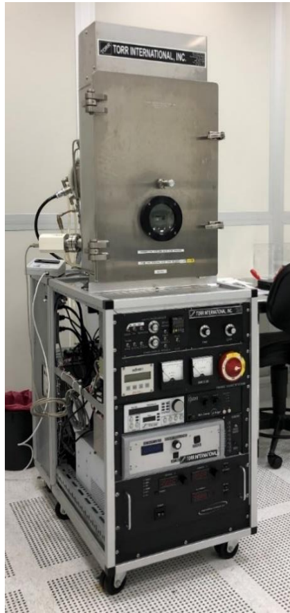
Figure 16 Torr International Evaporator.
