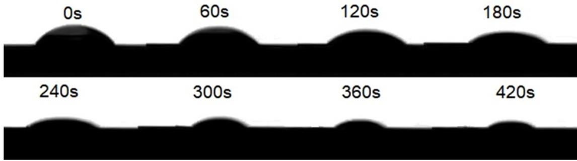
Figure 4.1 Evaporation of water droplet on SiO<sub>2</sub> substrate
