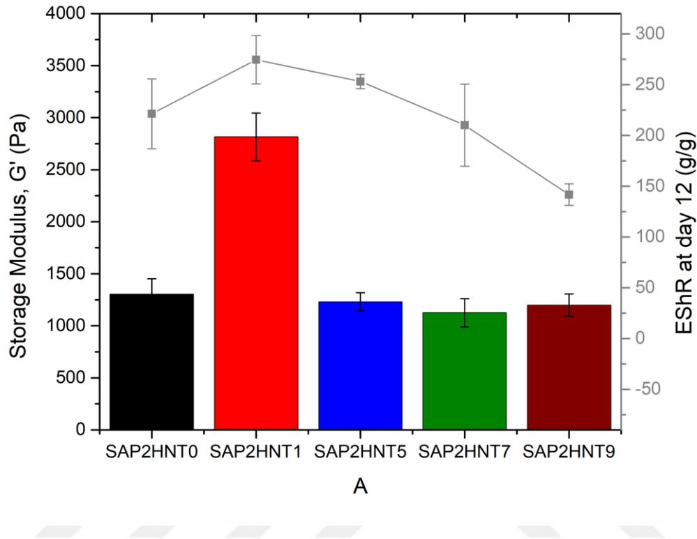
**Figure 3.6** Storage modulus results of SAP and SAP-HNT Nanocomposites
