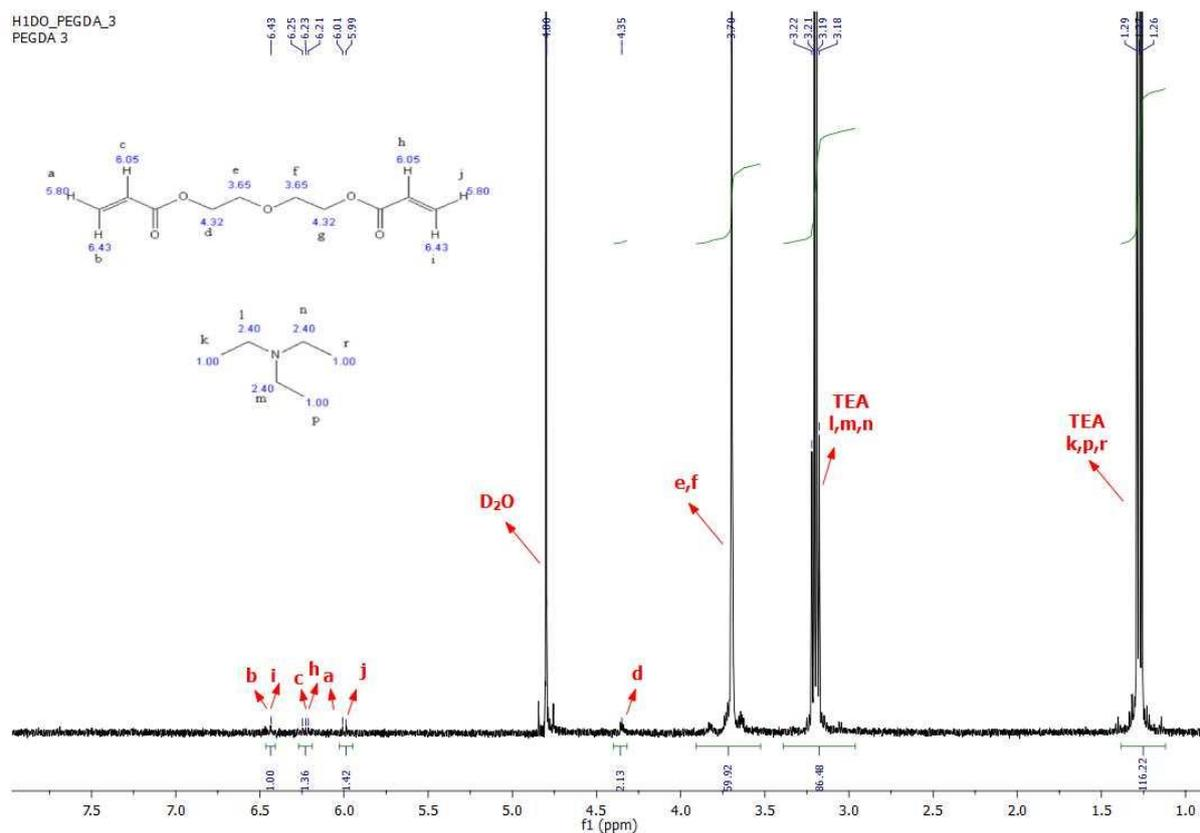
**Figure 4.2** Proton NMR spectrums of PEGDA1 (a), PEGDA2 (b), and PEGDA3 (c) synthesized crosslinker monomer
