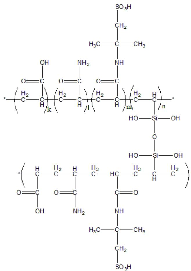
**Figure 2.1**The reaction and crosslinking mechanism of SAP2HNT0
