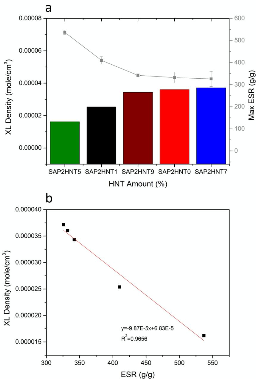
**Figure 3.4** Maximum swelling ratios of SAP2 dataset polymers in water (a), crosslink density as a function of ESR (b).
