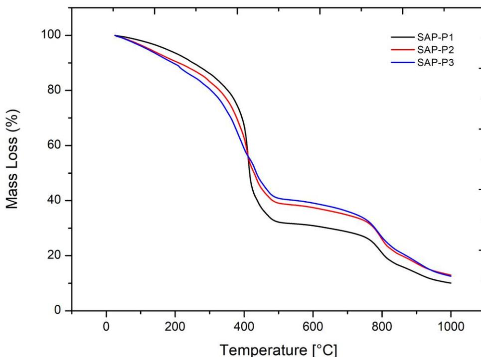
**Figure 4.8** TGA curves for SAP-Px under nitrogen atmosphere
