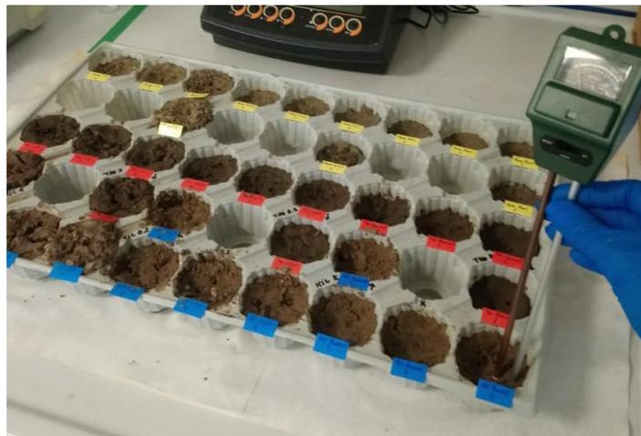
**Figure 3.7** The experimental setup of loamy, clay, and sandy soil with control, 0.5% and 5% SAP doses(a) and procedure of soil moisture measurement with moisture probe (b)
