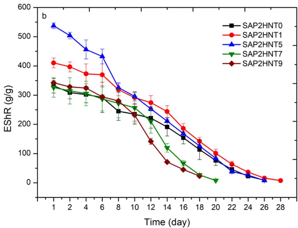
**Figure 3.3** The swelling (a) and water-release (b) test results of SAP2 polymer set involving different amounts of HNT
