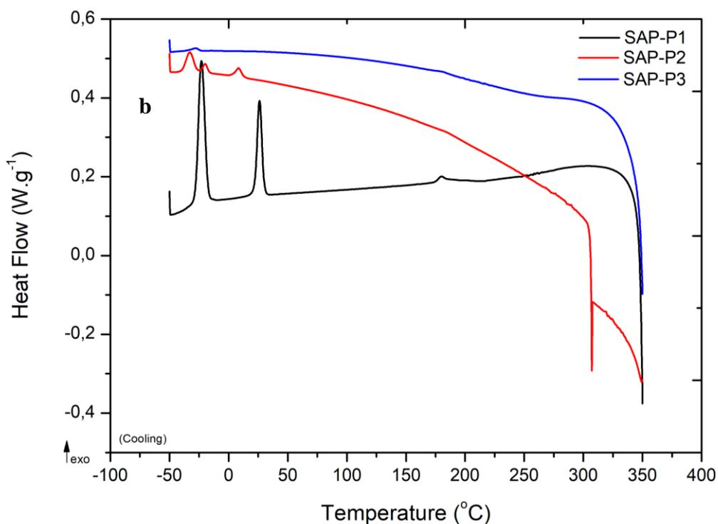
**Figure 4.9** First heating (a) and cooling (b) DSC curves for SAP-Px data set under nitrogen atmosphere
