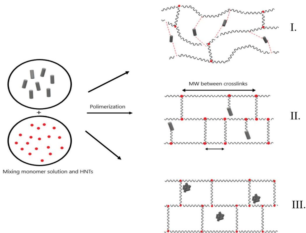
**Figure 3.5** The graphical representation of three different HNT incorporation mechanisms into SAP nanocomposite structure
