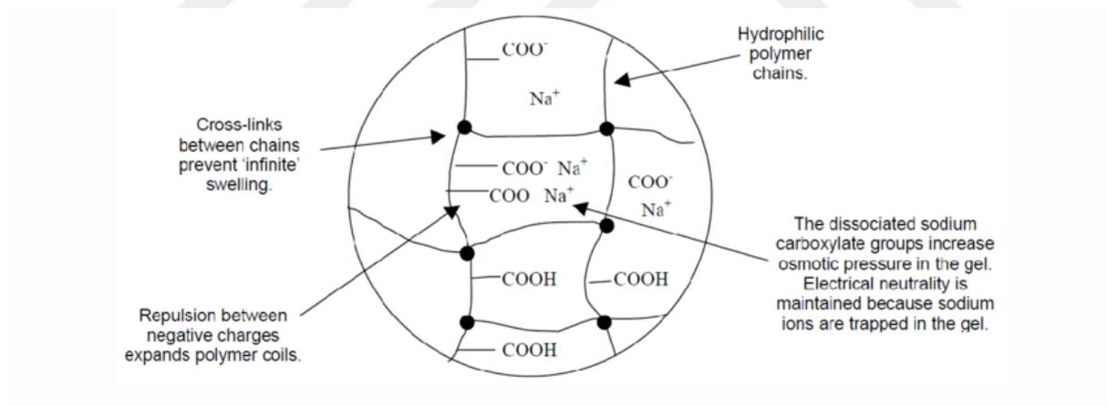
**Figure 1.1** The swelling mechanism of super-absorbent polymers [34]
