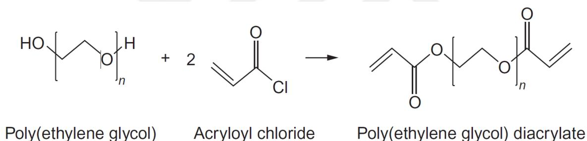
**Figure 4.1** The reaction mechanism of PEGDA monomer synthesis
