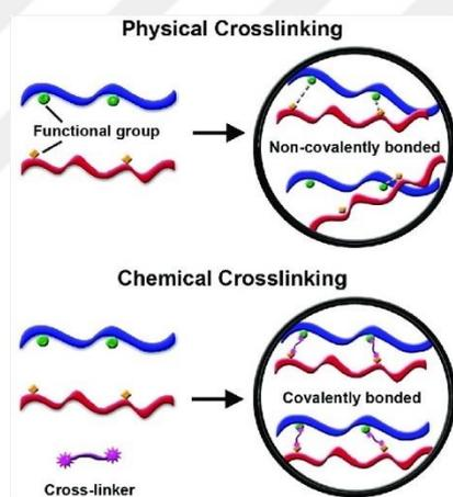
**Figure 1.3** The graphical representation of physical and chemical crosslinking mechanisms [38]
