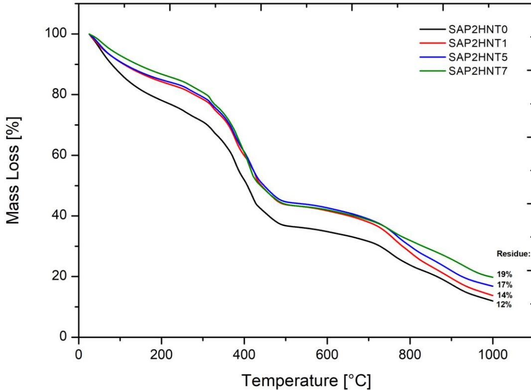
**Figure 3.2** Thermogravimetric analysis of SAP and SAP-HNT nanocomposites
