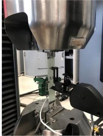
Figure 35 Tensile test setup
