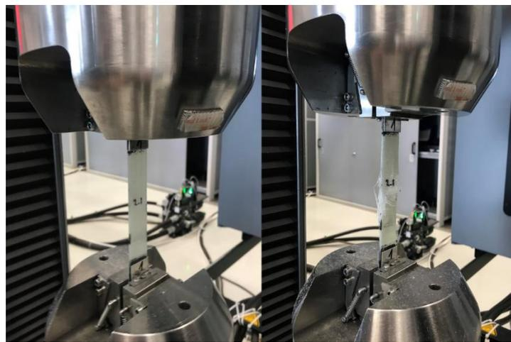
Figure 36 Tensile test specimen before (left) and after (right) tensile test
