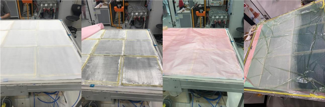
Figure 32 Steps of vacuum infusion process
