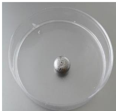
Figure 44 Fe 50 Pt 50 alloy fabricated by arc melting
