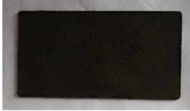
Figure 8 1 mm thick NdFeB slice cut by EDM
