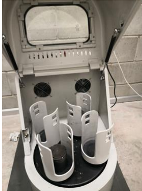
Figure 10 MTI Corporation SFM-1 Planetary Ball Milling Instrument
