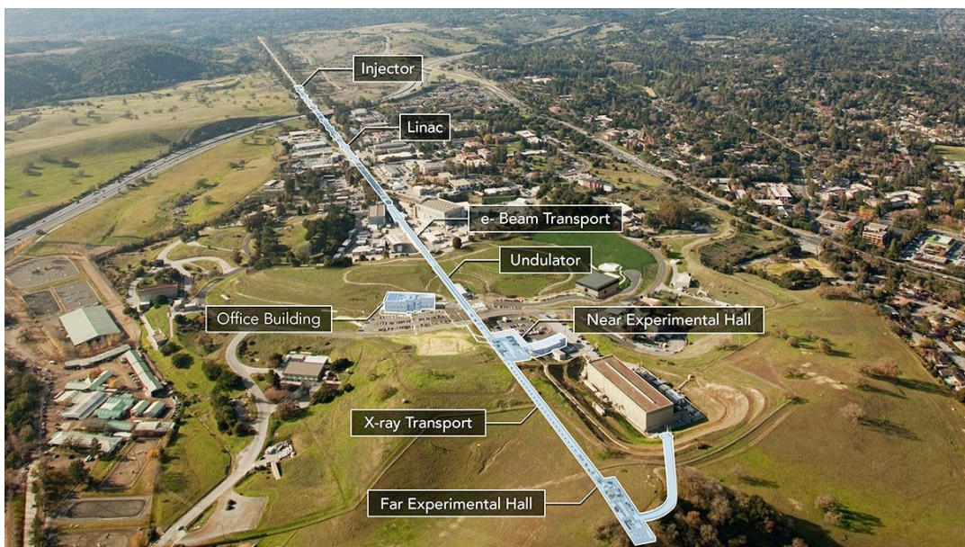
Figure 2 The bird's eye view of LCLS/SLAC (3.2 km length)
