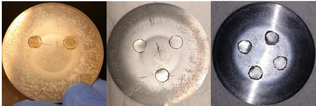
Figure 18 Hybrid FePt targets with 2 Pt pieces (left); 3-Pt pieces (middle); 4-Pt pieces (right)
