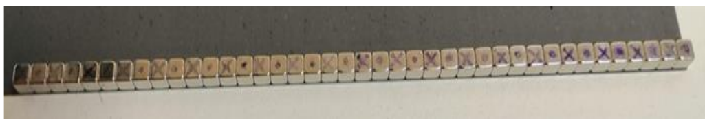
Figure 11 Set of 3 mm cubic NdFeB magnets mounted in Up-Down array
