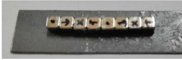
Figure 12 Set of 3 mm cubic NdFeB magnets mounted in Halbach array
