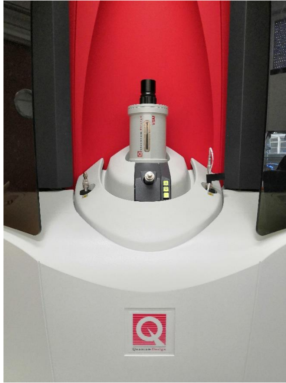
Figure 28 Quantum Design MPMS 3, VSM-SQUID instrument
