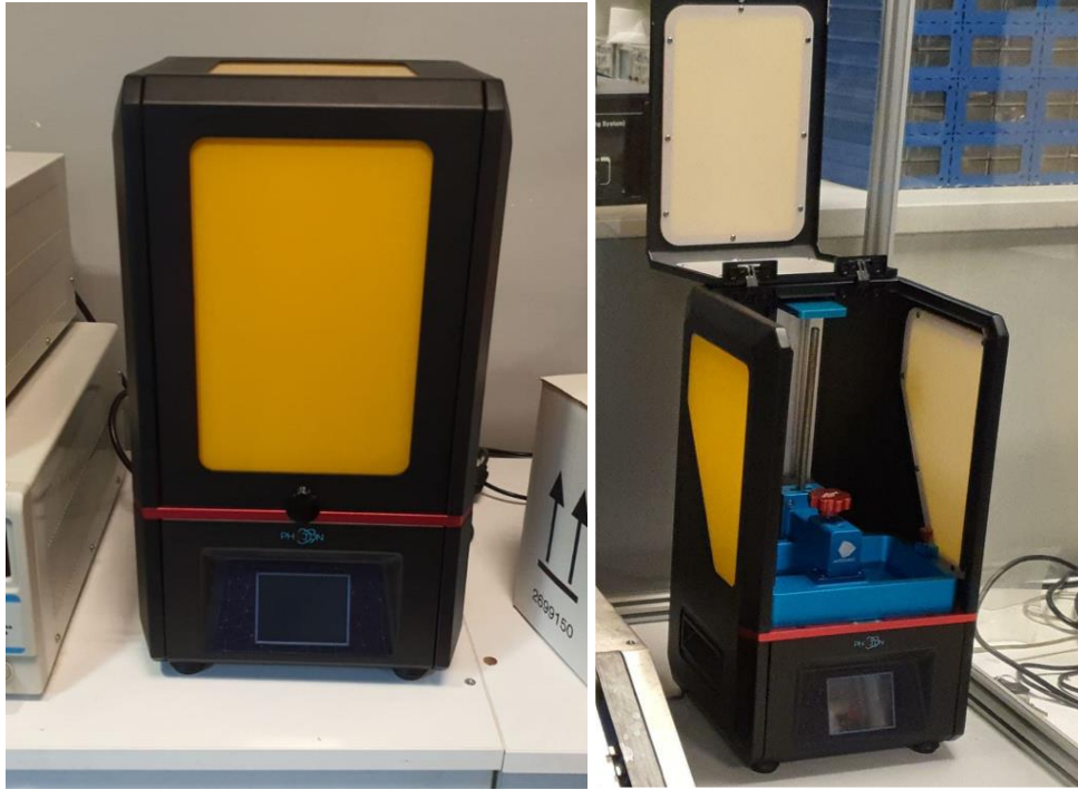
Figure 14 Anycubic Photon LCD-based SLA 3D Printer instrument
