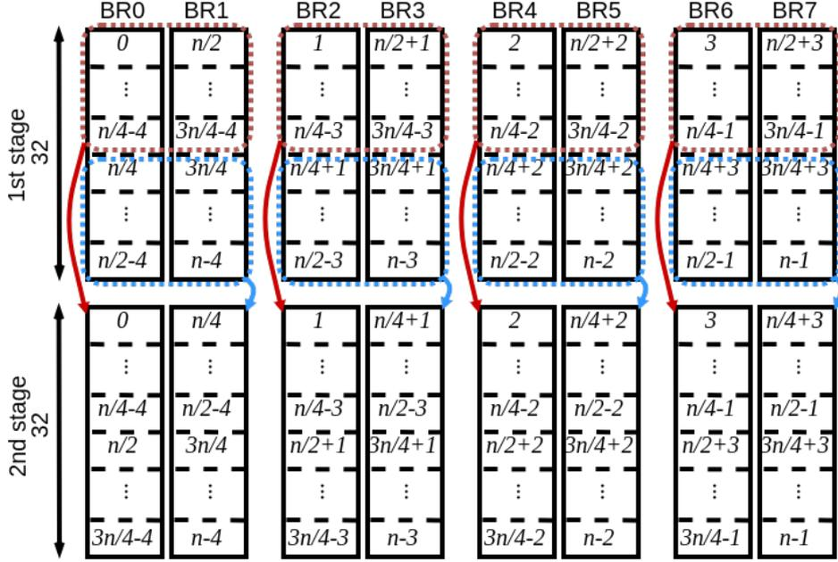
Figure 6.6 Memory Access Pattern for four Butterfly Units
