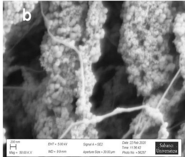
Figure 3-11. Electrospun matrix of \text{TiO}_2/\text{CB}/\text{Polymer}=70/20/10 with PEO solid ratio of 5% and PR=5: 22 % ink solid ratio.
